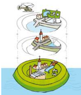
Figure 7.1. Multi-Layer Safety; from bottom to top: 1) prevention; 2) land use planning; 3) evacuation and emergency response. (Figure courtesy of Rijkswaterstaat)
