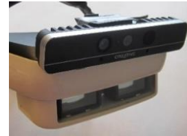
Fig. 3. Cinoptics AIRO II HMD for AR with the Intel® RealSense F200 mounted on top of it.
