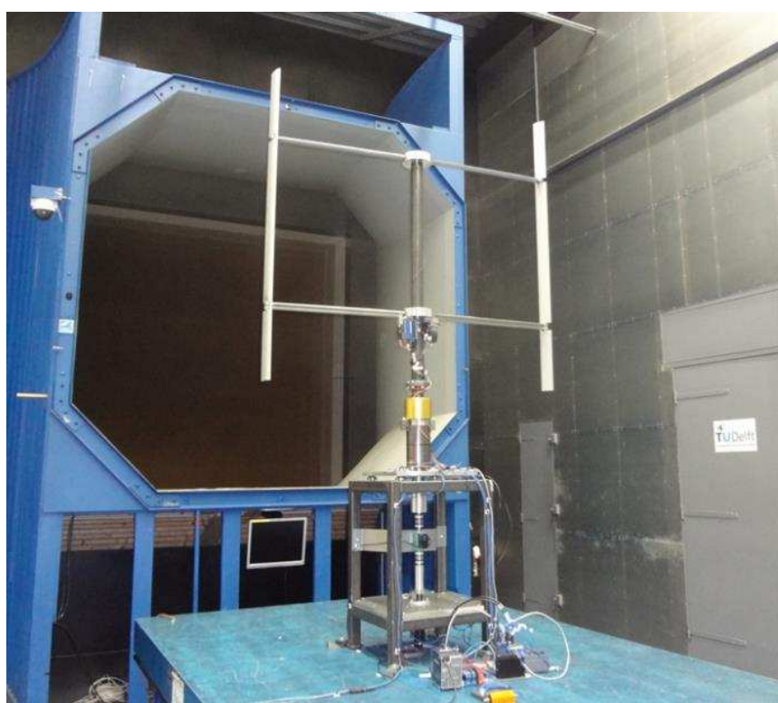
Figure 1. Test setup and sample results for PitchVAWT Wind Tunnel Testing at TU Delft Facilities.
