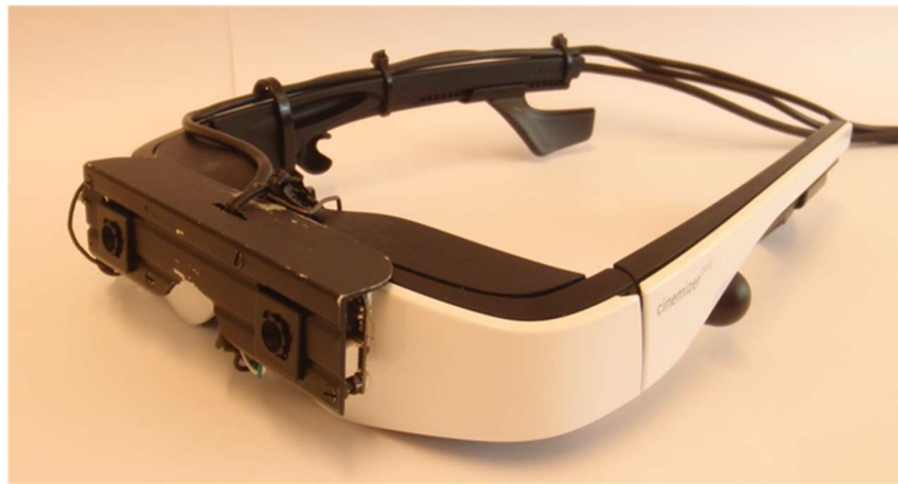
FIGURE 49 THIRD ITERATION OF THE HARDWARE FOR VIDEO SEE-THROUGH
