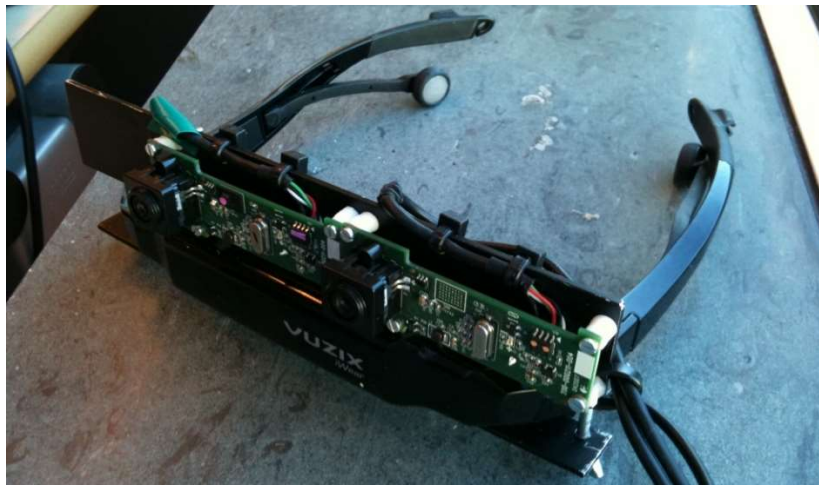
FIGURE 47 FIRST ITERATION OF THE HARDWARE FOR VIDEO-SEE THROUGH
