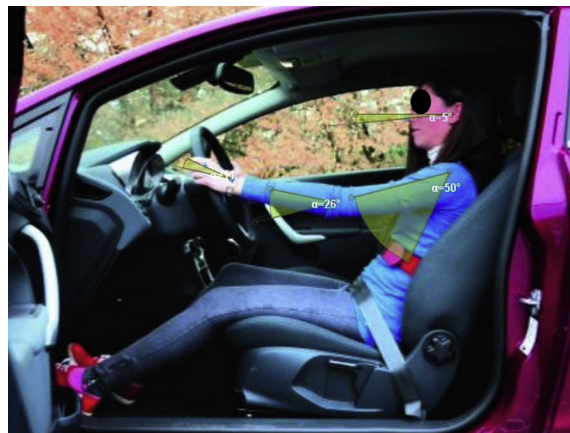
Fig. 3.13: First Driving Posture: car seat far from dashboard
