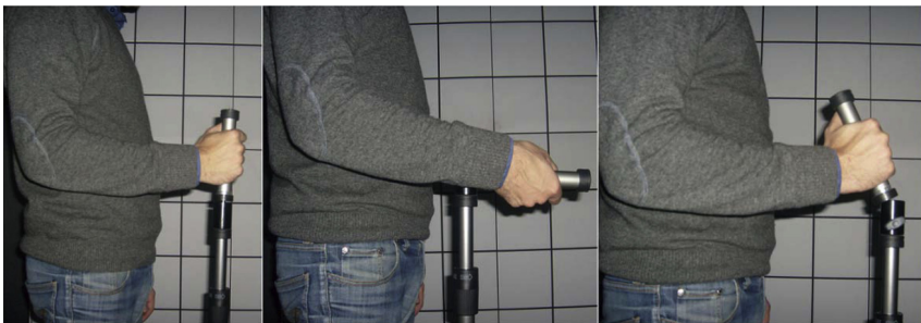
Fig. 3.7: Wrist joint – Radio-Ulnar Deviation test
