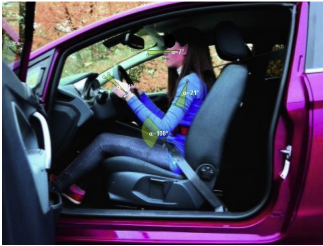
Fig. 3.14: Second Driving Posture: car seat close to dashboard
