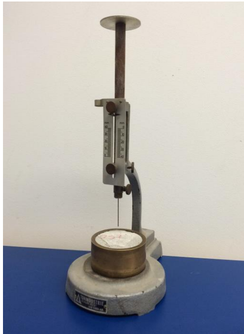
Figure 3:2: Vicat apparatus for determination of setting time, which is measured as the penetration behaviour of a standard needle in a cement (fly ash) paste.
