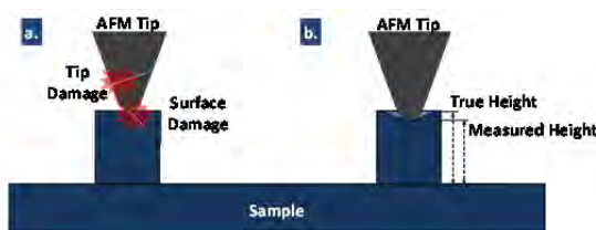
Fig. 1: Surface and/or tip damage during imaging (a) or hindering the true height measurement of sample structures (b).
