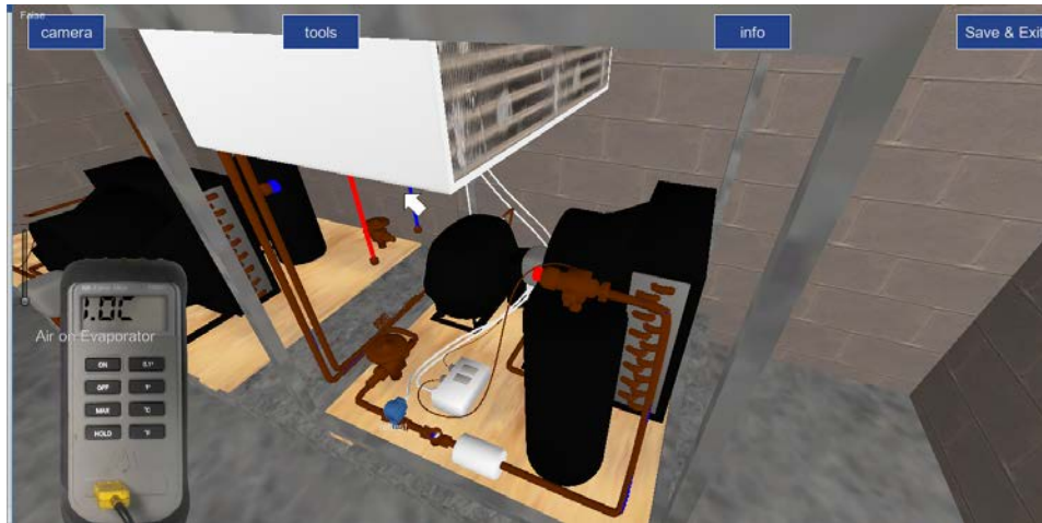
Figure 5.16: 3D modelled evaporator and thermometer object measuring air on temperature
