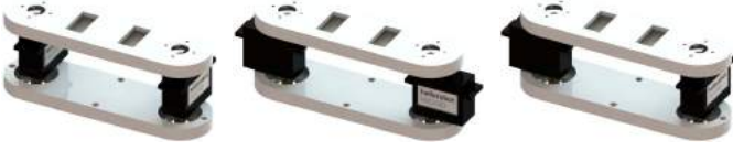
Fig. 5. Examples of possible orientations of two HX1218D servomotors for driving the link. Rotation axes of servomotors coincide with the rotation axes of boxes, and the link connecting two servomotors must be perpendicular to rotation axes. In our design, the link is hollowed such that electric wires connecting the male and female boxes can be placed inside.
