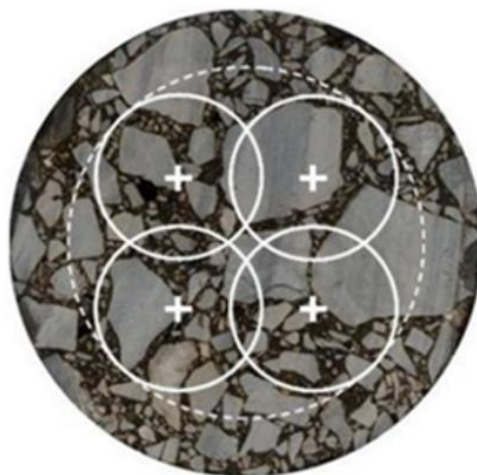
Figure 2. Thermal parameter test points of specimen.
