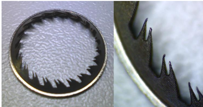
Figure 3.7. Prototyped steel teeth ring, using tooth geometry J (Figure 3.6, bottom), 2.0 mm height, 1.4 mm width, 0.3 mm spacing between teeth, and 45° inward angle. The ring has 21 teeth.
