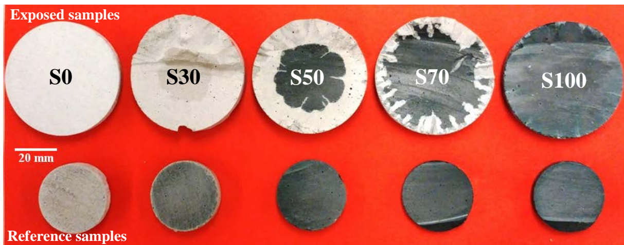
4 Fig. 2. Cross-sections of representative samples after natural laboratory carbonation of 1 year, 5 clearly showing the outer (carbonated) and the inner (noncarbonated) zone. Reference 6 samples are of smaller diameter, placed beneath the exposed samples.
