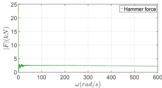
Fig. 3. Frequency spectrum of the hammer force
