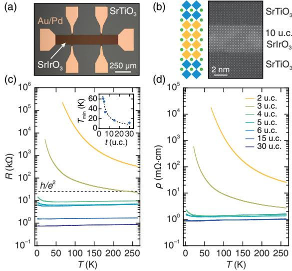
FIG. 1. (a) Optical image of a Hall bar used for transport measurements. (b) HAADF-STEM image of a SrTiO<sub>3</sub>/10 u.c. SrIrO<sub>3</sub>/SrTiO<sub>3</sub> heterostructure. (c)  $R(T)$  and (d)  $\rho(T)$  curves for films of different thicknesses. The inset shows the temperature of the resistance minimum ( $T_{\min}$ ) as a function of thickness.
