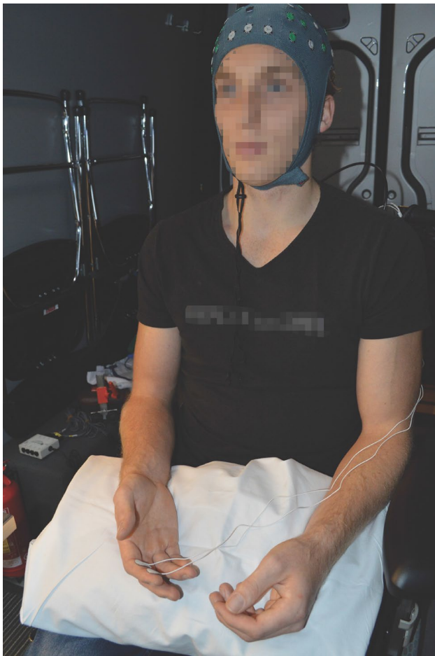
Fig. 1 Experimental setup. One participant is seated on a wheelchair inside the experimental van with his dominant hand on a supine position, placed on a pillow. Here, the electrodes are attached on his index finger
