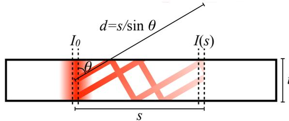
Fig. 2. The two rays drawn are both emitted at an angle  $\theta$  from different depths within the LSC. Both rays have to travel the same distance  $s / \sin(\theta)$  to reach a column at a distance  $s$ , viewed from the top of the LSC. The radiant power  $I(s)$  of the light from both rays is therefore equal at  $s$ , independent of the depth the light was emitted from.
