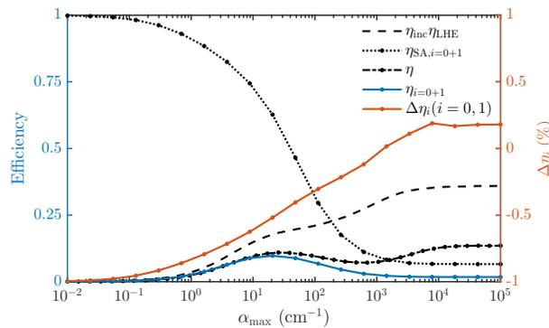
Fig. 7. Optimization track of a  $10 \times 10 \times 0.5 \text{ cm}^3$  Red305 LSC with  $\eta_{\text{QV}} = 1$ . A second maximum is seen in the optical efficiency. Here the second MGLT generation contributes more to the edge-transmission than the first generation.
