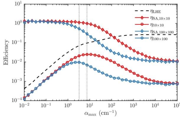
**Fig. 5. Optimization track for GQD ( $\eta_{\text{QV}} = 0.45$ ) using two different LSC sizes.** The displayed efficiency is the total optical efficiency, calculated through MC. Dotted lines indicate the maxima for the two simulated geometries.
