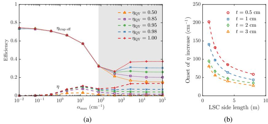
Fig. 6. (a) Optical efficiency  $\eta$  (dashed) and effective trapping efficiency  $\eta_{\text{trap eff}}$  (dotted) in Red305 for increasing quantum yields. The white area indicates the region with low optical density, and the shaded area indicates high optical density. (b) Onset of the increase in  $\eta$  for  $\eta_{\text{QY}} = 1$  Red305 LSCs of varying sizes and thicknesses. This onset is defined as the point where  $\eta$  starts rising again. Lines are drawn as a guide to the eye.
