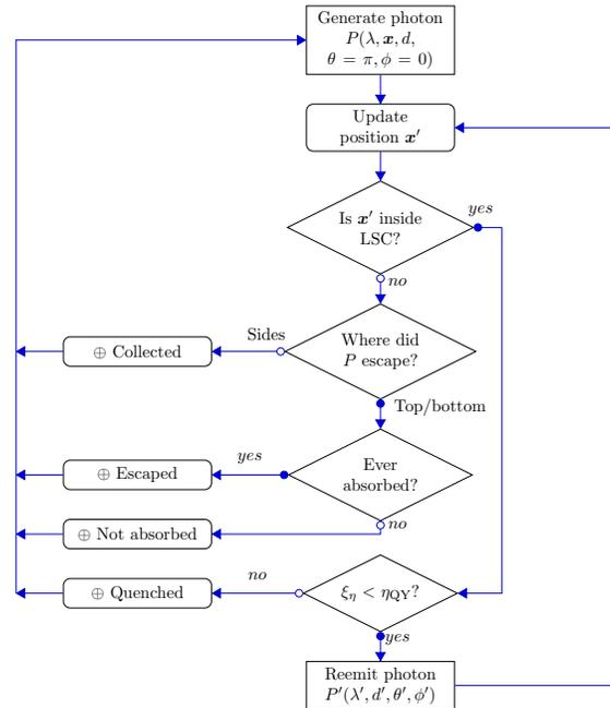
Fig. 3. Schematic representation of the MC simulation.
