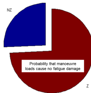
Figure 2.10: Pie chart showing an example of how probable it is that there are load cycles within a particular flight regime above the endurance limit (Z) or not (NZ).
