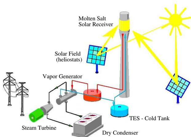
Fig. 1. Schematic layout of the Gemasolar 20 MW<sub>el</sub> (15 hours of storage) solar tower plant, adapted from Burgaleta et al. (2011).
