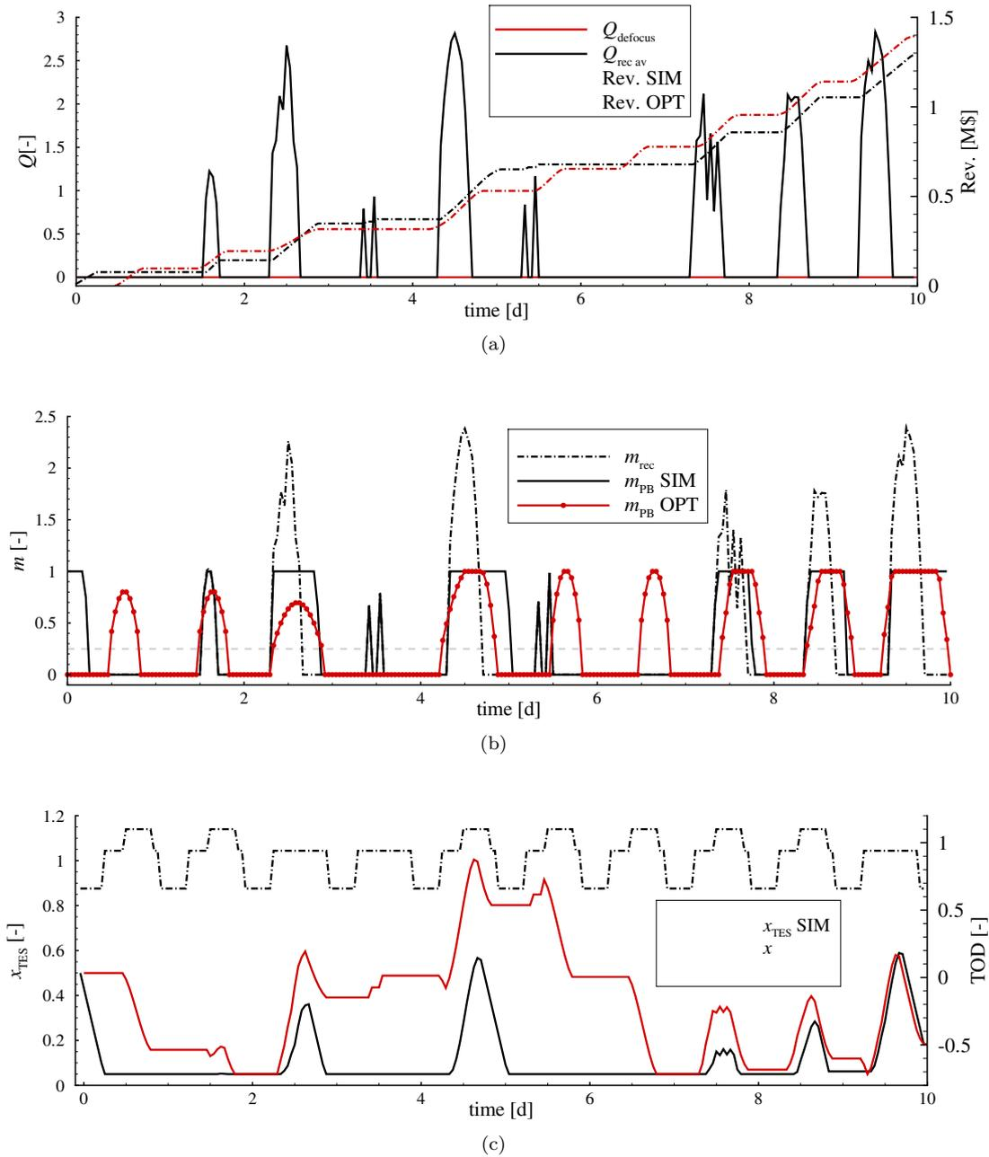
Fig. 2. Comparison between reference and optimized operation for a solar tower plant during a 10-days period from February the 7<sup>th</sup> to February the 16<sup>th</sup> (location Daggett - CA, weather data in the TMY2 format). The considered system features solar multiple  $SM = 2.5$  and storage capacity  $T_{\text{TES}} = 15$ .
