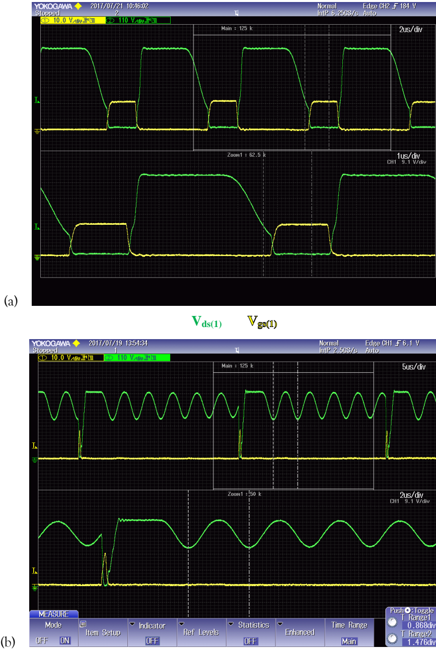
Fig. 5.15. Drain-source voltage V_{ds} and gate voltage V_{gs} for one phase of the IBFC for CH mode: (a) Quasi-resonant operation LVS for V_{ev}=250V , I_{ev}=5A (b) Valley skipping and DCM operation at low powers for V_{ev}=100V , I_{ev}=1A
