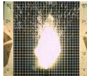
5-kJ pyrotechnical igniter
