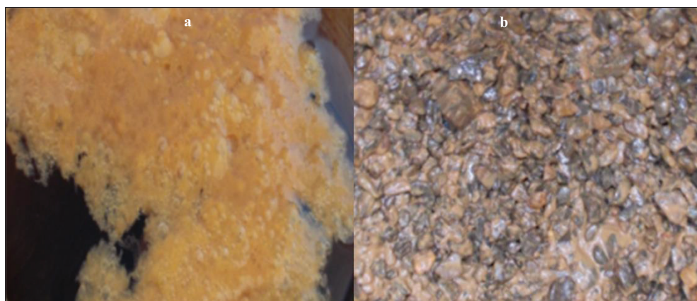
Figure 5.8. Photograph of Fe in the form of gelatinous agglomerates in line at low oxygen concentrations: (a) at the inlet of F1 and (b) in the gravel media of F1.
