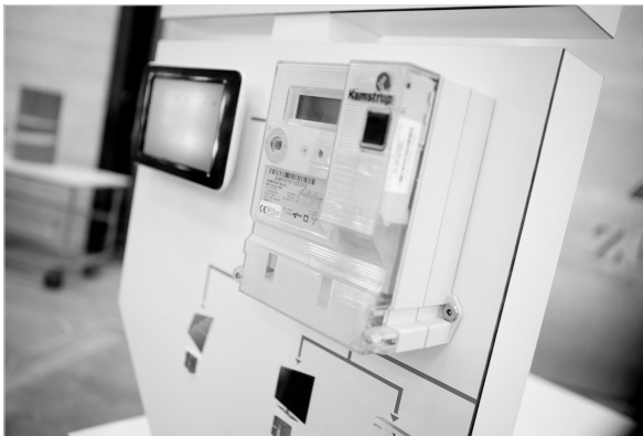
FIG.1.5 EXAMPLE OF A SMART METER CONNECTED TO A COMPUTERISED FEEDBACK DEVICE
