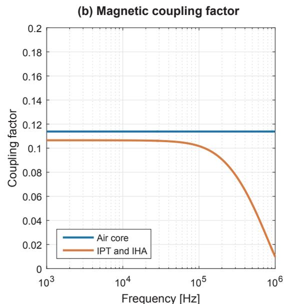
Fig. 8. Performance of a combined IPT and IHA system compared with an air core system. (a) Shows the maximum efficiency from the primary to the secondary and (b) shows the magnetic coupling factor between the primary and secondary.
