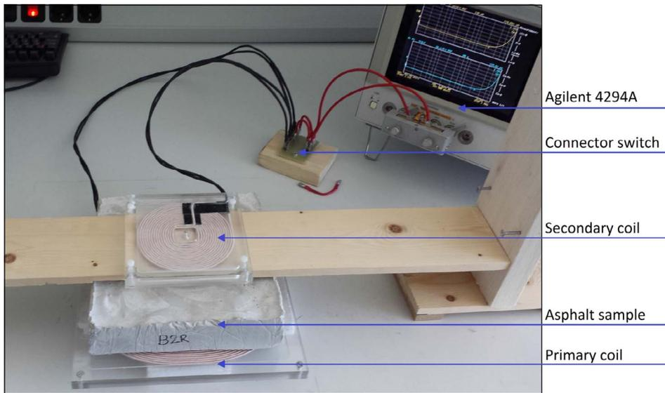
Fig. 10. Overview of the setup of the measurement of combined IHA-IPT with a rectangular block of asphalt.
