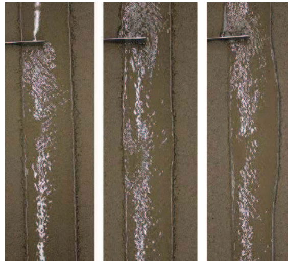
Figure 15. Channel-width evolution after 0 (left), 8 (middle), and 16 (right) hours.
