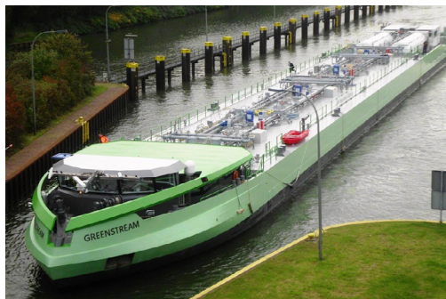
Figure 4-16. The Greenstream: The first 100%, LNG-powered inland shipping vessel
