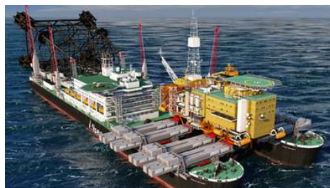
Figure 4-7. The Pioneering Spirit: A split bow platform decommissioning vessel
