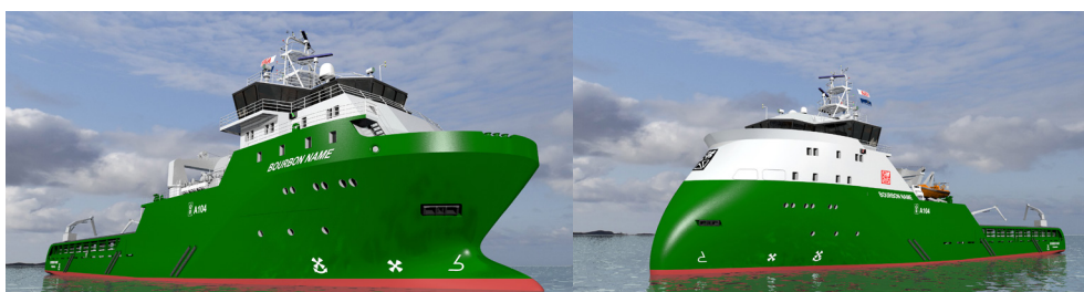
Figure 4-21. Status January 2005, both the conventional bow (left) and the X-bow® (right)
