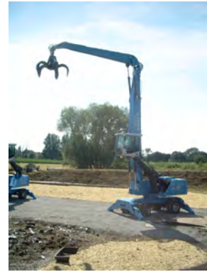
(c) Hydraulic grab. Copyright Strominski.
