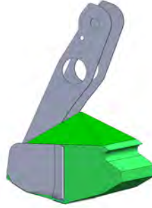
Figure 8.3: Definition of maximum capacity of grab V_{\text{grab}} .
