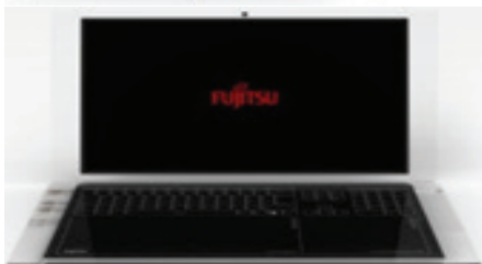
FIGURE A.22: PV-POWERED NOTEBOOK, BY FUJITSU (2011). IT IS A POLYCARBONATE LAPTOP WITH A TRANSPARENT TOUCH-KEYBOARD, WHICH HAS DOUBLE SOLAR PANELS (ONE ON TOP AND UNDER THE KEYPAD). © ANDREA PONTI. SOURCE: YANKODESIGN, 2011.
