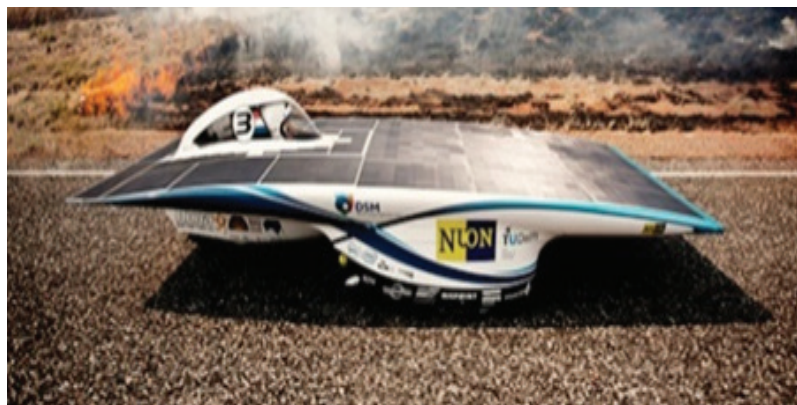
FIGURE 1.14: NUNA 3 SOLAR-POWERED RACING CAR, BUILT BY TECHNICAL UNIVERSITY OF DELFT, IN THE NETHERLANDS, 2004-2005 (NUON SOLAR TEAM, 2015). PHOTO BY HANS-PETER VAN VELTHOVEN.
