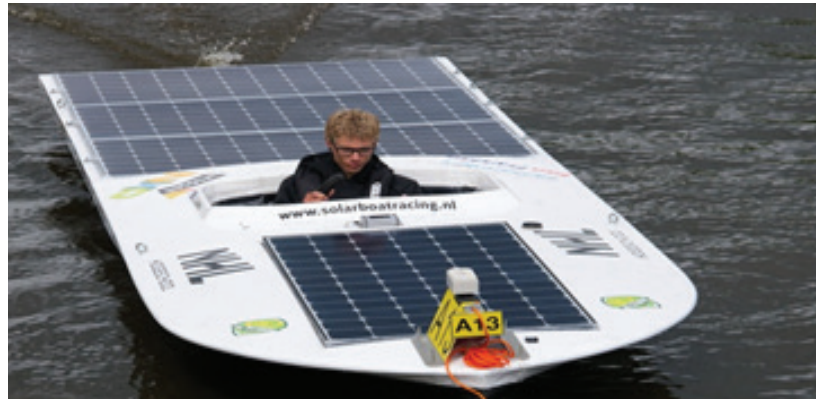
FIGURE 1.16: THE PV-POWERED A-BOAT AT THE NHL SOLARBOAT RACING (GORTER, 2014).
