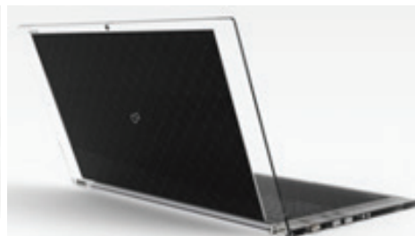
FIGURE A.22: PV-POWERED NOTEBOOK, BY FUJITSU (2011). IT IS A POLYCARBONATE LAPTOP WITH A TRANSPARENT TOUCH-KEYBOARD, WHICH HAS DOUBLE SOLAR PANELS (ONE ON TOP AND UNDER THE KEYPAD). © ANDREA PONTI. SOURCE: YANKODESIGN, 2011.
