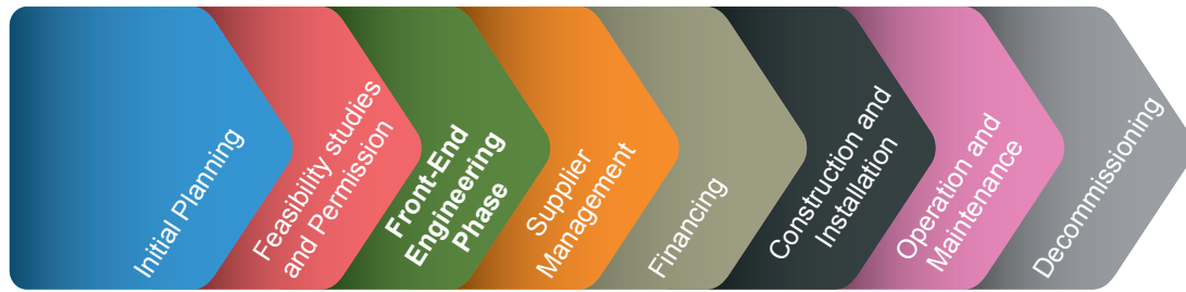
Figure 5.2: Lifecycle of an OWF and location of the FEED phase [14, 17].
