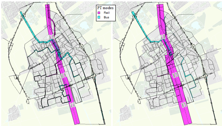
Figure 2.9. Average public transport flows (h -1 ) between 17:30 and 18:00 for the Delft case study on a normal day (left) and in the evacuation scenario (right). Bar widths are proportional to flow, colours indicate public transport mode.
