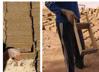
FIGURE 2.20 Traditional method for casting mud brick, still used in few places, Dakhla oasis, Egypt
