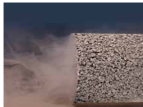
FIGURE 4.45 Air Permeable Concrete by Ole Daniels and Jesper Nørgaard at Aalborg University
