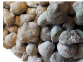
FIGURE 4.44 APC sample by the author showing voids formation
