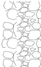
FIGURE 2.2 Section in old traditional stone external wall
