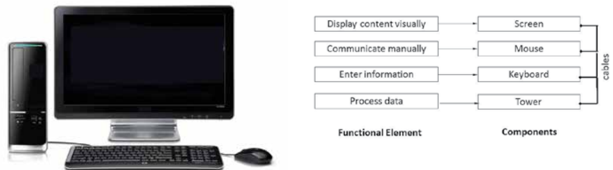
FIGURE 3.3 Modular product architecture of a desktop computer
