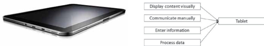
FIGURE 3.4 Integral product architecture of a tablet
