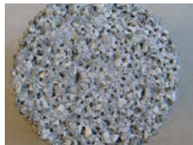
FIGURE 4.45 Air Permeable Concrete by Ole Daniels and Jesper Nørgaard at Aalborg University
