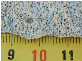
FIGURE 4.21 Air cells of Aerated Concrete
