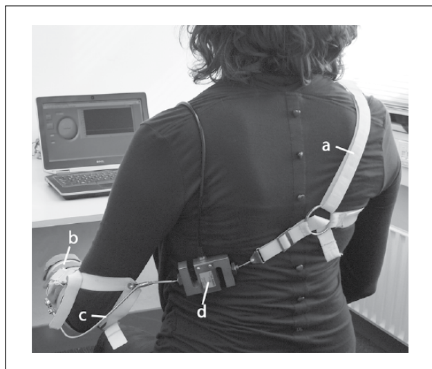
Figure 1. Measurement setup for maximum force measurements: (a) the “figure-of-nine” harness and (b) thermoplastic shell are connected through a (c) Bowden cable, which is interrupted by a (d) force sensor. In this setup, cable excursions are disabled.
