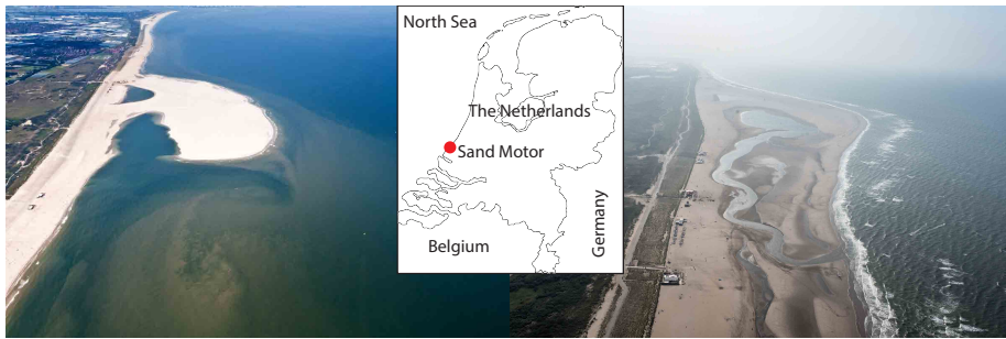
Figure 3.1: The Sand Motor mega-nourishment in the Netherlands (left) just after construction in 2011, with turbidity patterns at the sea surface revealing signs of a separating tidal flow field, and (right) in 2014, after approximately 3 years of morphological development. Images by Joop van Houdt / Rijkswaterstaat.
