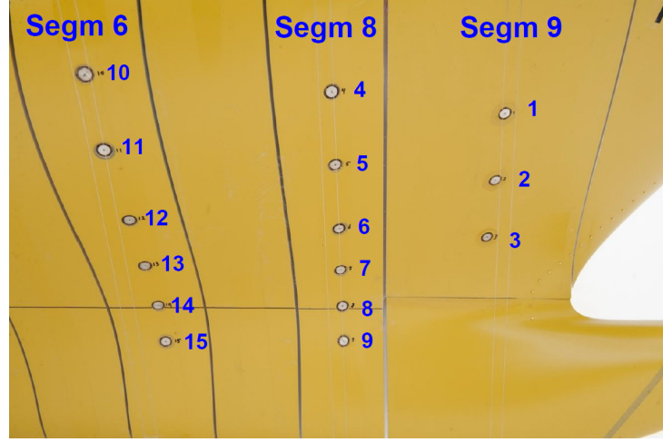
Figure 4.9: Pressure sensors on the windward side of the segmented model. The rows are vertical and located on St\ 17.89 , St\ 18.77 and on St\ 19.50 . The horizontal levels are -1.472 , 0.039 , 1.547 , 3.051 , 5.055 and 7.050 m relative to the undisturbed water surface. The row at St\ 19.50 has the sensors only at the top 3 positions.
