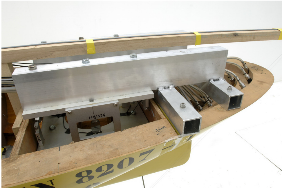
Figure 4.4: Force balance to measure the forces on the bow segment. The force is transferred from the bow segment to the 6-component frame through the large size aluminium beams fitted in longitudinal direction. The 6-component frame is fitted underneath these beams on the left hand side. The force sensors are protected during handling by vertical plates - these are still fitted in the picture.
