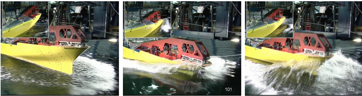
Figure 8.10: Stills from the video of the experiments, the start of the impact at t = 101 s, the maximum immersion of the model and the moment the spray drops back in the water.
