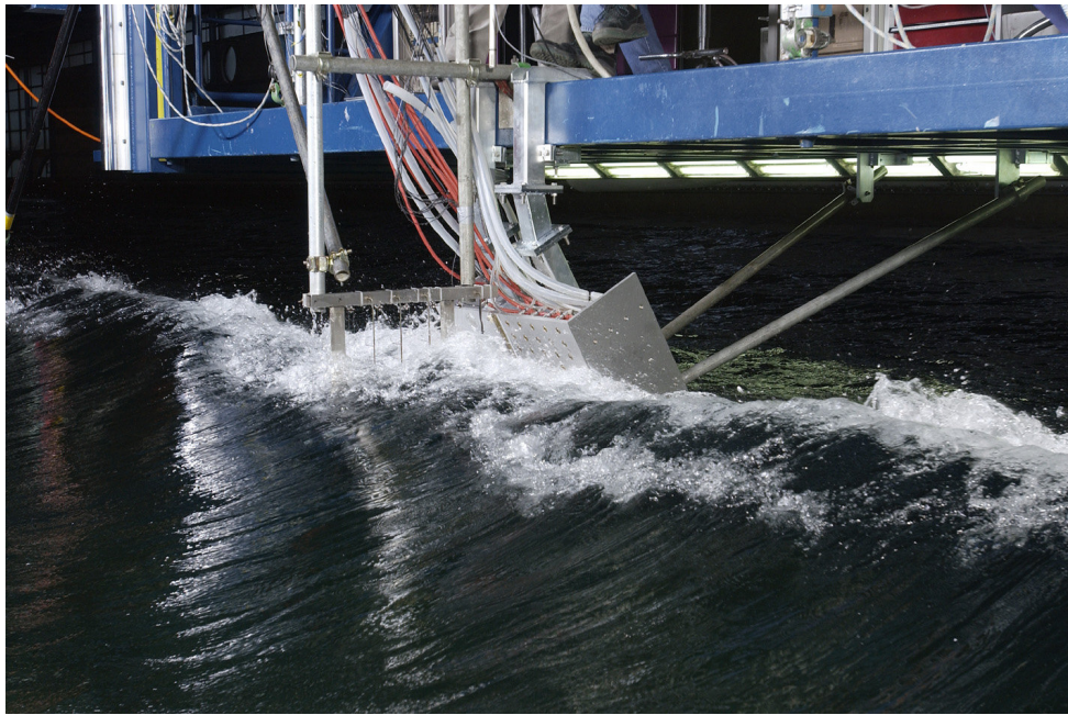
Figure 5.36: Measurement of wave slap load due to a breaking wave. The picture is taken just before the impact.
