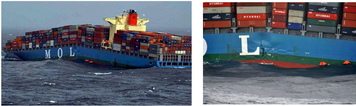
Figure 1.3: The container vessel MOL Comfort broke her back in 2013.
