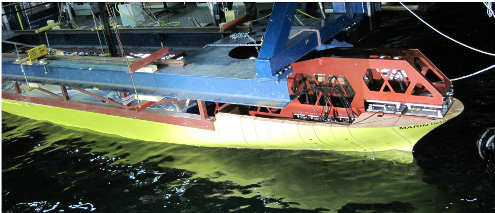
Figure 4.8: Model of the ferry in the Seakeeping and Manoeuvring Basin. Captive set-up.
