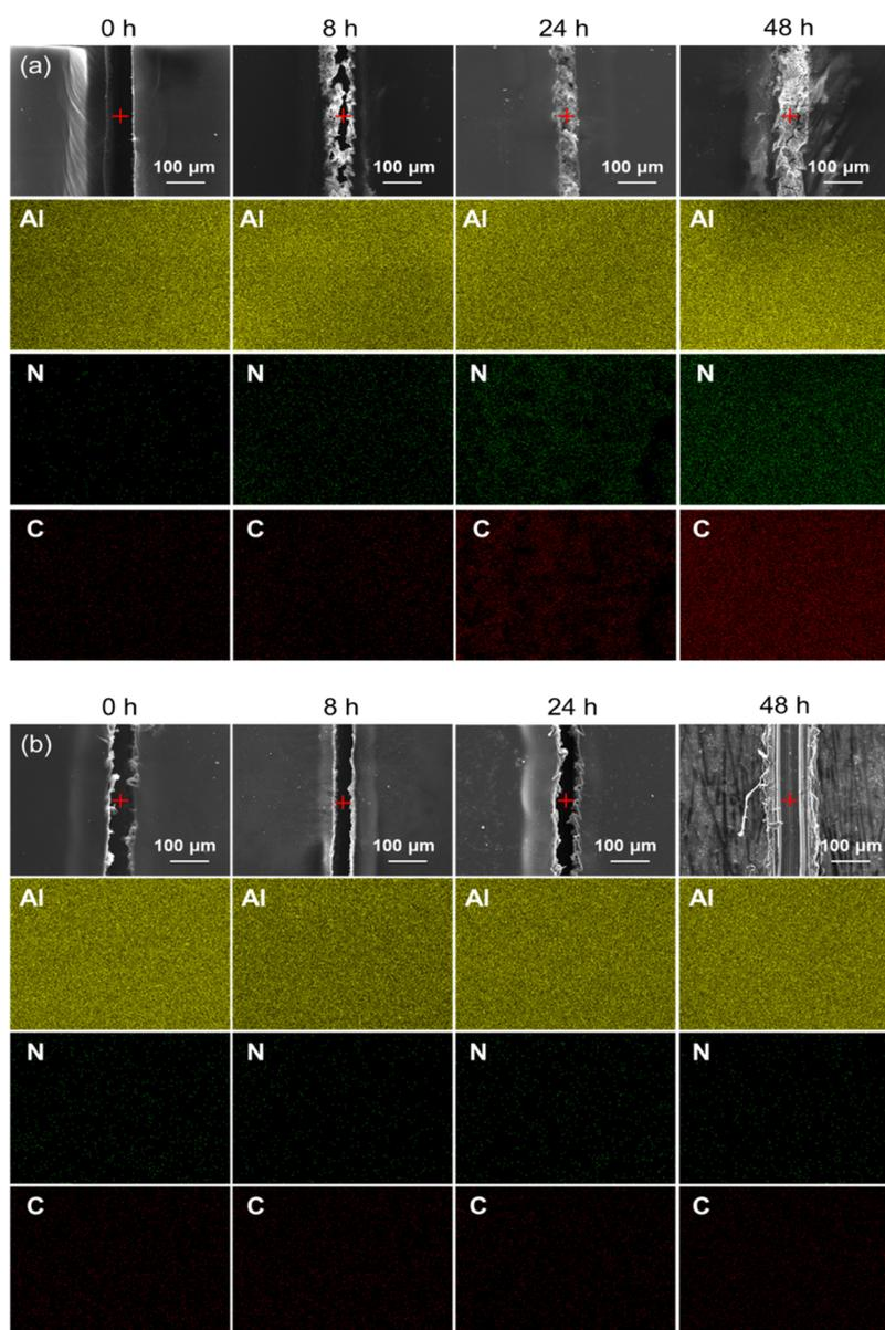
**Figure 7.** EDS maps in the scratched area of (a) coatings with 10 wt % 8HQ–PCL and (b) 10 wt % PCL microspheres after immersion in 3.5 wt % NaCl for 0, 8, 24, and 48 h. The EDS map was taken over an area of  $2 \times 1.6 \mu\text{m}^2$  at the location indicated by the red cross in the SEM image.
