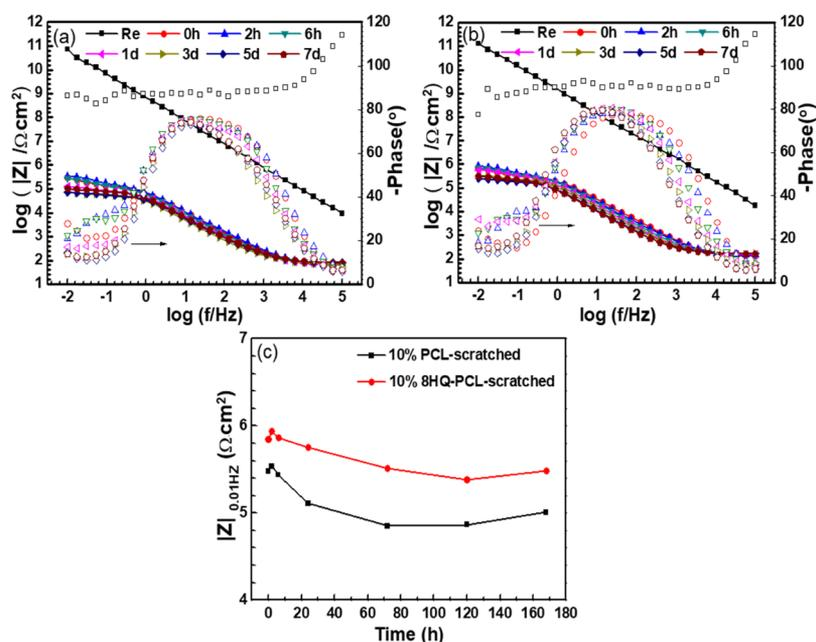
**Figure 6.** Bode plots of (a) scratched coatings with 10 wt % PCL microspheres and (b) scratched coatings with 10 wt % 8HQ–PCL microspheres after 0, 2, and 6 h and 1, 3, 5, and 7 d of immersion in 3.5 wt % NaCl solution; (c) comparison between  $|Z|_{0.01\text{Hz}}$  values for scratched coatings with 10 wt % 8HQ–PCL microspheres and 10 wt % PCL microspheres. Closed symbols represent impedance modulus values, and open symbols show phase angles.
