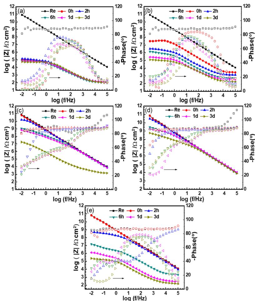
**Figure 5.** Evolution of Bode plots of the scratched coatings immersed in 3.5 wt % NaCl solution for 3 days: (a) blank SMP coating before heating, (b) heated blank SMP coating, (c) heated coating with 5 wt % PCL microspheres, (d) heated coating with 10 wt % PCL microspheres, and (e) heated coating with 15 wt % PCL microspheres. The closed symbols represent impedance modulus values, and the open symbols indicate phase angles.
