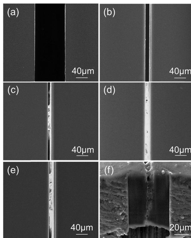
**Figure 4.** SEM images of the self-healing coating surfaces: (a) originally scratched surface, (b) heated blank SMP coating, (c) heated coating with 5 wt % PCL microspheres, (d) heated coating with 10 wt % PCL microspheres, (e) heated coating with 15 wt % PCL microspheres, and (f) FIB-prepared cross section of the healed scratch area of the coating with 10 wt % PCL microspheres.
