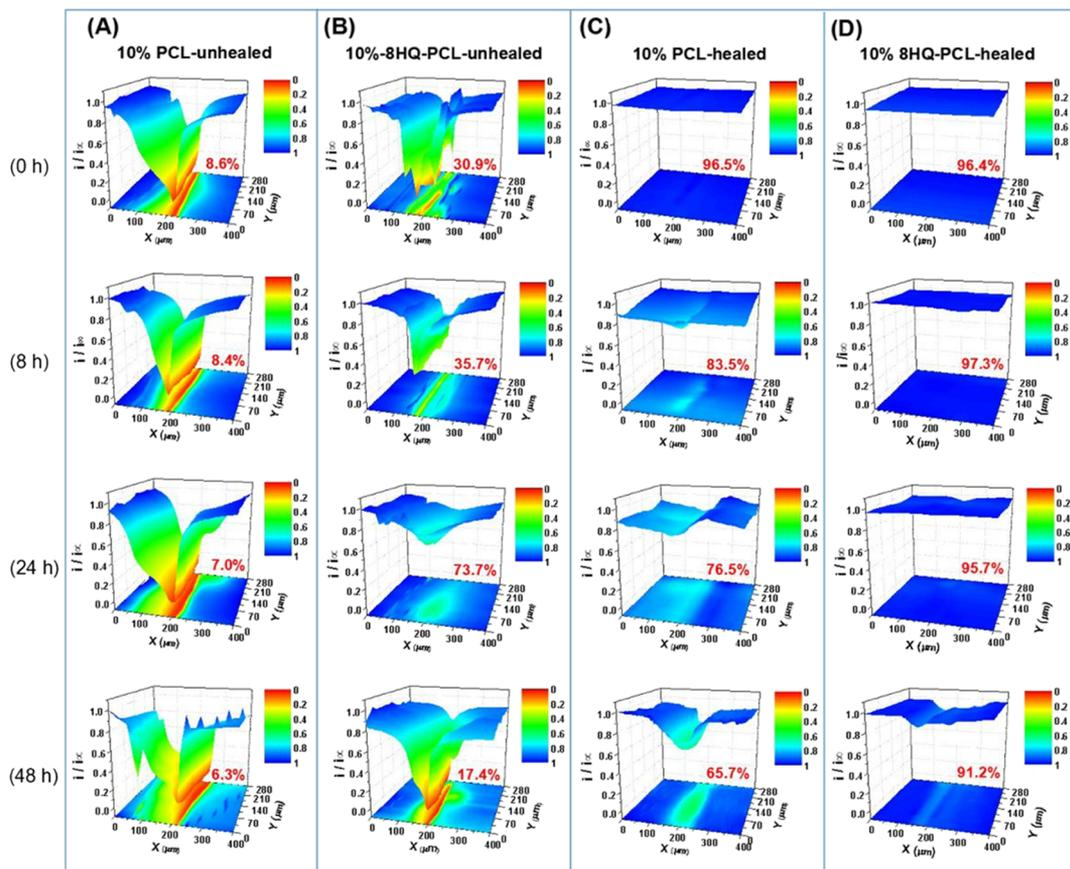
**Figure 10.** SECM maps of the scratch regions on (a) scratched coatings with 10 wt % PCL microspheres, (b) scratched coatings with 10 wt % 8HQ-PCL microspheres, (c) heated coatings with 10 wt % PCL microspheres, and (d) heated coatings with 10 wt % 8HQ-PCL microspheres after immersion in 3.5 wt % NaCl solution for 0, 8, 24, and 48 h.
