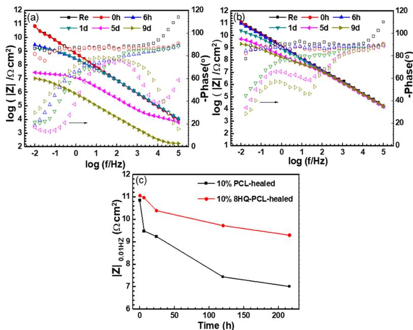
**Figure 9.** Bode plots of (a) heated coatings with 10 wt % PCL microspheres and (b) heated coatings with 10 wt % 8HQ-PCL microspheres after 0 and 6 h and 1, 5, and 9 d of immersion in 3.5 wt % NaCl solution; (c) comparison between  $|Z|_{0.01\text{Hz}}$  values for heated coatings with 10 wt % 8HQ-PCL microspheres and 10 wt % PCL microspheres. The closed symbols represent impedance modulus values, and the open symbols indicate phase angles.
