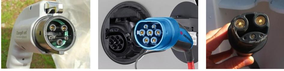
Fig. 1. Plug for AC charging- US Type 1 SAE (left), European Type 2 Mennekes (middle) and Tesla plug (right)<sup>1</sup>
