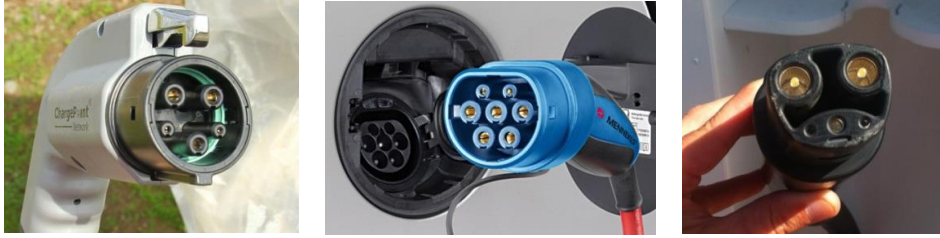
Fig. 1. Plug for AC charging- US Type 1 SAE (left), European Type 2 Mennekes (middle) and Tesla plug (right) 1
