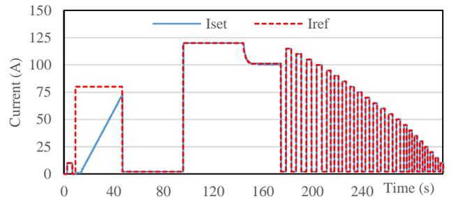
Fig. 8. Measurement of charger current reference  $I_{ref}$  sent every 100ms over PLC and corresponding EV current request  $I_{set}$  for CCS compatible EV of manufacturer 1 (top) and manufacturer 2 (bottom).
