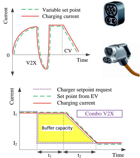
Fig. 5. Dynamic charging and V2X using CCS/COMBO (top) and the required buffer capacity (bottom)
