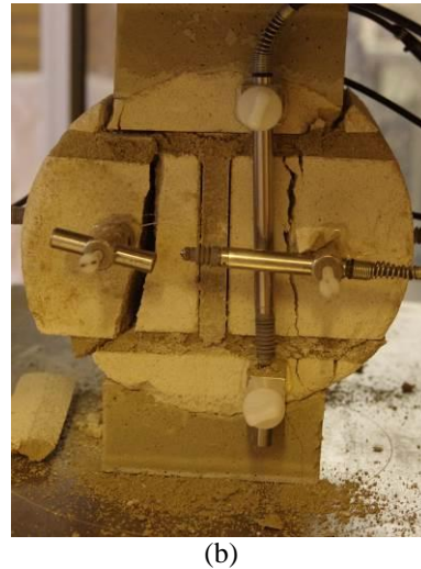
Figure 3: Splitting tests on masonry cores : (a) stress-strain curve; (b) typical observed crack pattern.
