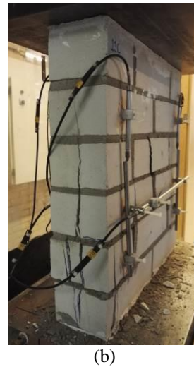
Figure 4: Compression tests on the companion masonry wallets: (a) stress-strain curve; (b) typical observed crack pattern.
