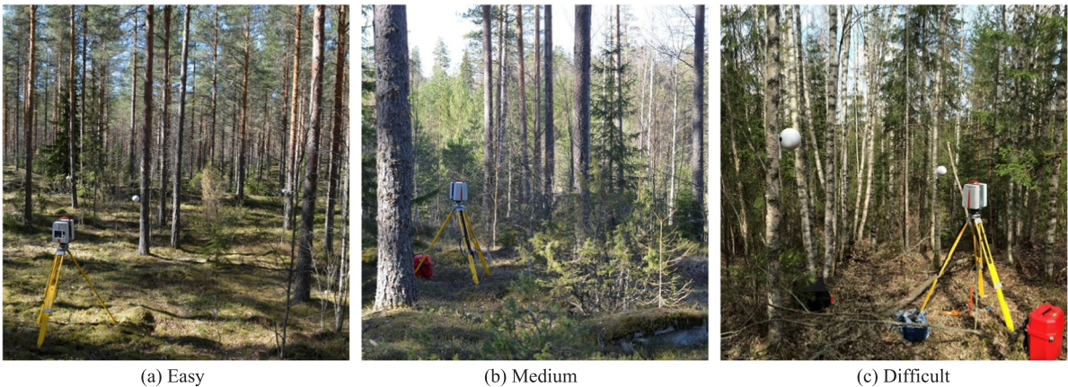
Fig. 3. Three complexity categories of the sample plots in the TLS benchmarking. The category “Easy” represents lower stem densities and little understory vegetation, “Medium” represents moderate stem densities and sparse understory vegetation, and “Difficult” represents high stem densities with dense understory vegetation.
