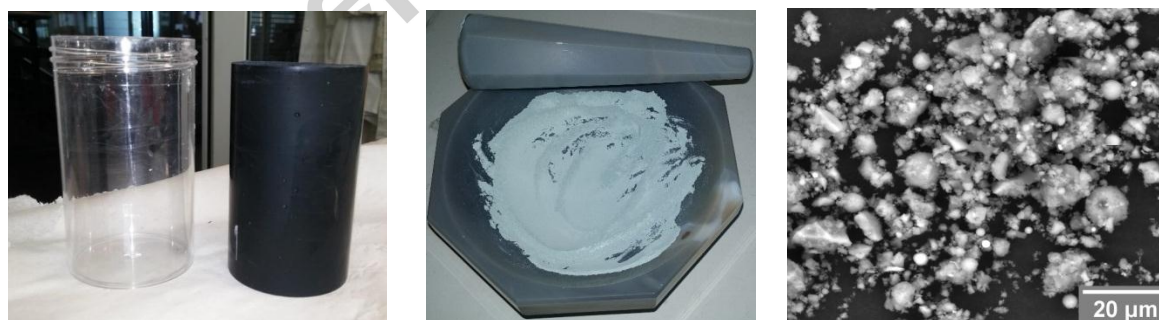
Fig. 2. Bulk sample after demoulding (left), ground sample (middle), SEM-BSE image of the powder (right).
