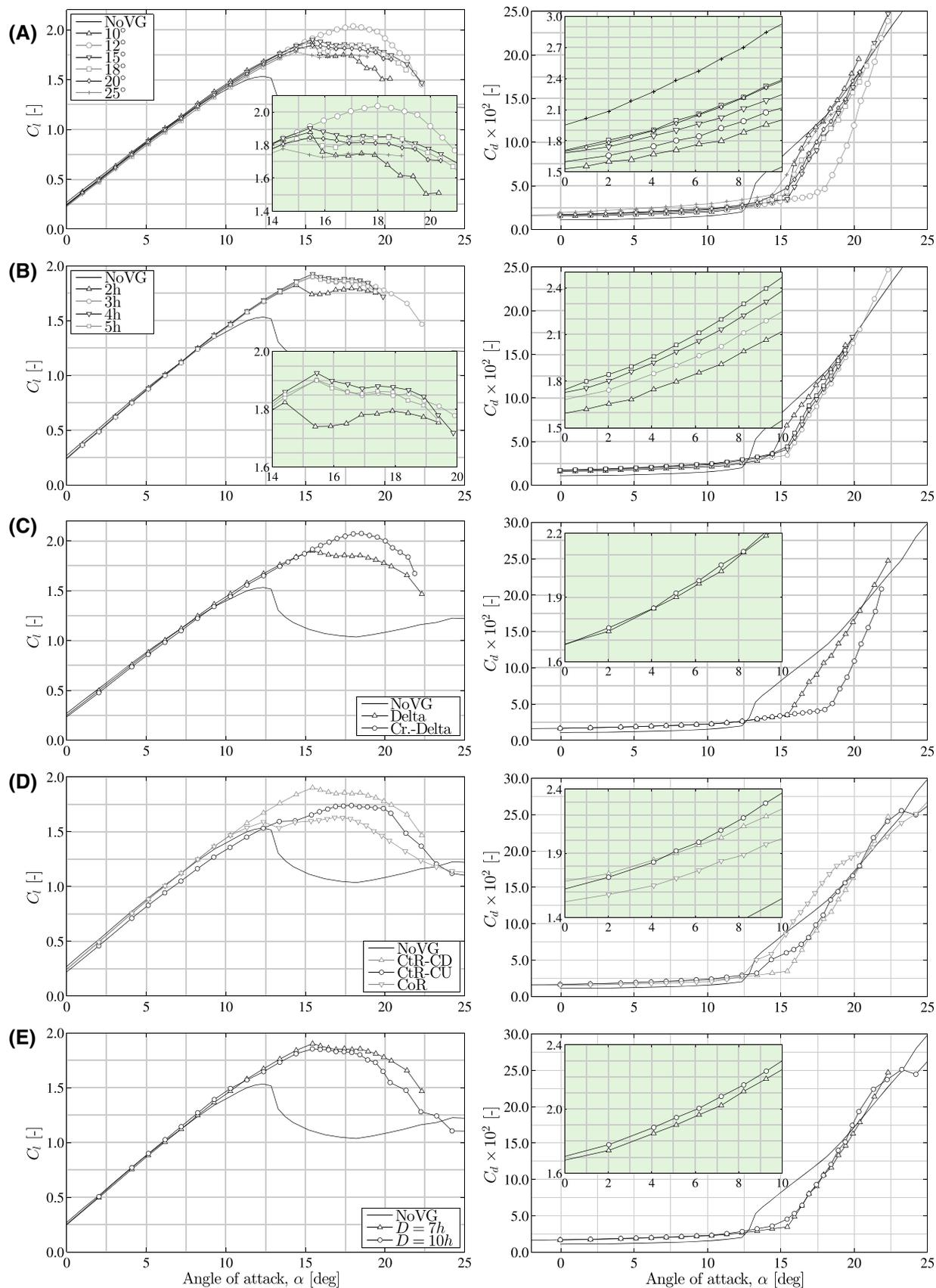
**FIGURE A3** Airfoil performance sensitivity to the A, vane angle; B, vane length; C, vane shape; D, array configuration; and E, pair spacing. CD, common downwash; CoR, corotating; Ctr, counter-rotating; CU, common upwash; NoVG, uncontrolled airfoil [Colour figure can be viewed at [wileyonlinelibrary.com](http://wileyonlinelibrary.com)]
