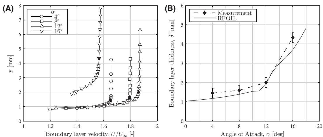
**FIGURE 7** A. Measured boundary layer profiles at  $x/c = 20\%$ . Filled black symbols indicate boundary layer edge; B, boundary layer thickness evolution with angle of attack. Case: clean, uncontrolled airfoil
