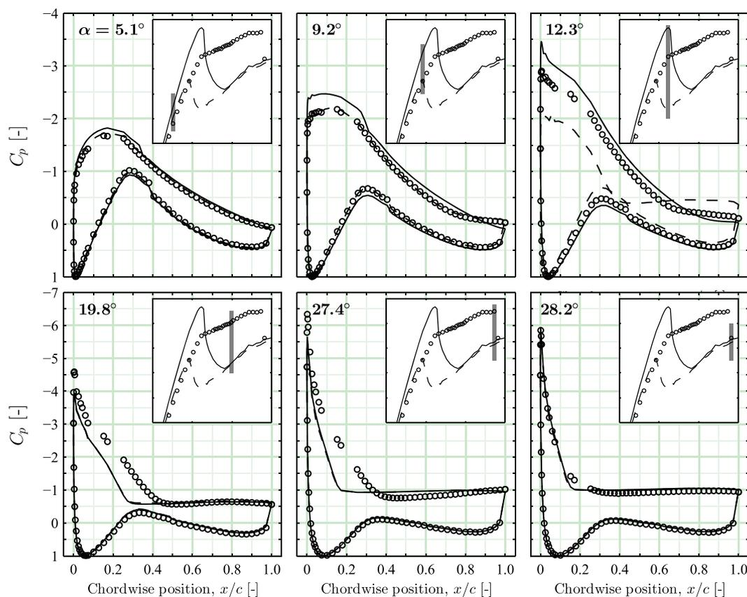
**FIGURE 15** Pressure distributions for increasing angles of attack, sampled along the lift polar as indicated in the inserts; clean (-) and rough (- -) uncontrolled cases; 2.5-mm VGs at  $x/c = 10\%$  in clean condition (o) [Colour figure can be viewed at [wileyonlinelibrary.com](http://wileyonlinelibrary.com)]
