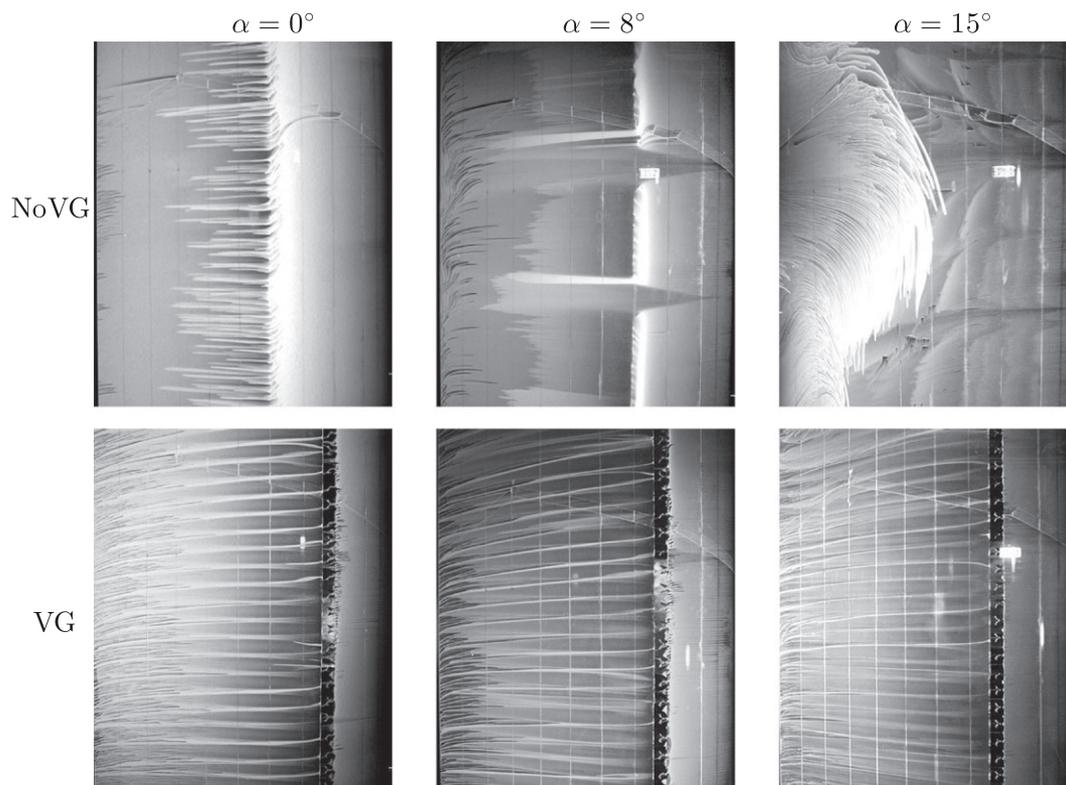
**FIGURE 8** Oil-flow visualization of the clean airfoil suction side for increasing angle of attack. Case: without and with (base design) vortex generators. Flow direction: right to left. NoVG, uncontrolled airfoil; VG, vortex generator
