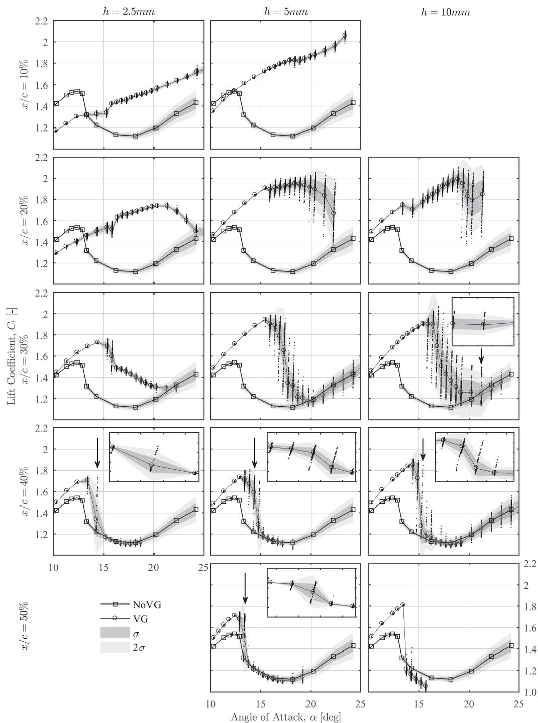
**FIGURE 18** Lift fluctuations for the uncontrolled and controlled cases with different vortex generator (VG) heights and chordwise positions. The solid lines and symbols are time-averaged measurements. Scattered data points show all observations in the sample, and the shaded bounds indicate deviations from the mean. Inserts centred about indicated positions (arrows) indicate bimodal behaviour. NoVG, uncontrolled airfoil
