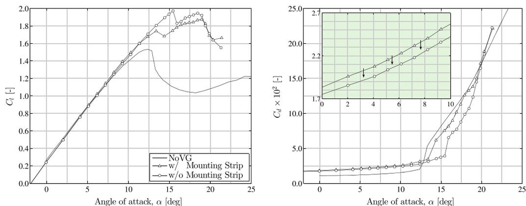
**FIGURE 13** Lift and drag polar showing the influence of the vortex generator mounting strip. NoVG, uncontrolled airfoil [Colour figure can be viewed at [wileyonlinelibrary.com](http://wileyonlinelibrary.com)]
