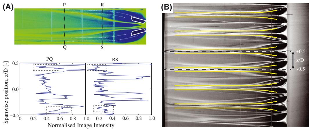
**FIGURE 9** A, Detailed oil-flow visualization over a spanwise period (top) with complimentary image analysis for vortex signature detection (bottom); B, visualization overlaid with predicted vortex paths (yellow dashed lines) in the streamwise-spanwise plane (Equations 3-4). Case:  $h = 10$  mm,  $x_{VG}/c = 20\%$ , airfoil suction side,  $\alpha = 0^\circ$  in free transition [Colour figure can be viewed at [wileyonlinelibrary.com](http://wileyonlinelibrary.com)]
