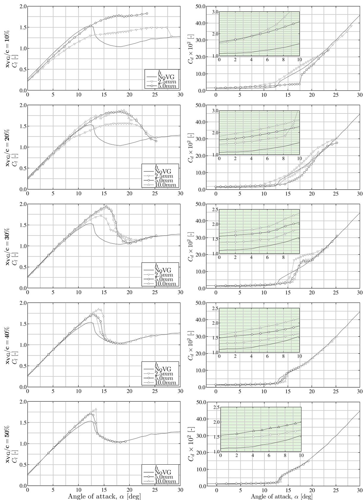
**FIGURE A1** Sensitivity to array chordwise placement and vortex generator vane height. Graphs are grouped into rows according to the array chordwise placement (top-bottom):  $x_{VG} = 10\%$  to  $50\%$ . NoVG, uncontrolled airfoil [Colour figure can be viewed at [wileyonlinelibrary.com](http://wileyonlinelibrary.com)]
