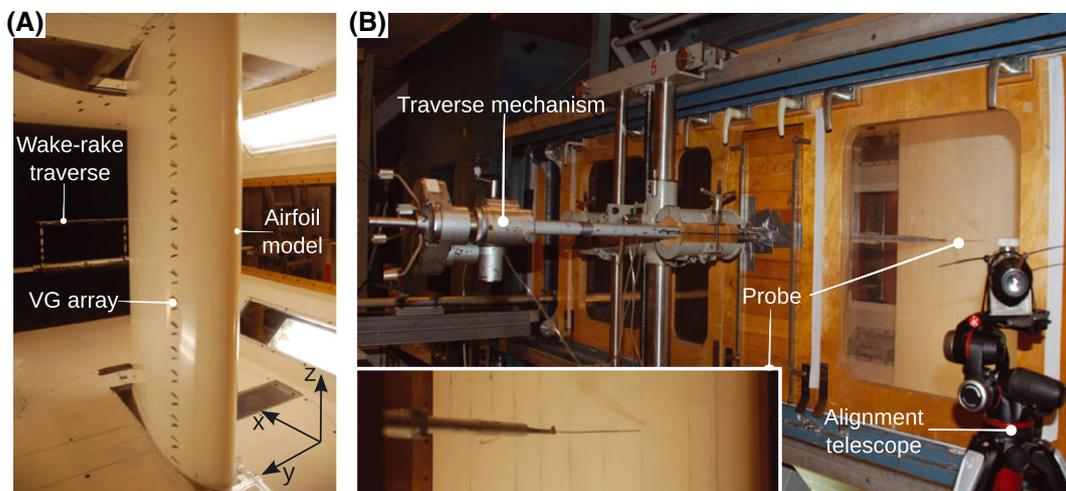
**FIGURE 5** A, Typical test-section setup showing the wake rake aft of the wing section; B, boundary layer measurement setup. VG, vortex generator [Colour figure can be viewed at [wileyonlinelibrary.com](http://wileyonlinelibrary.com)]
