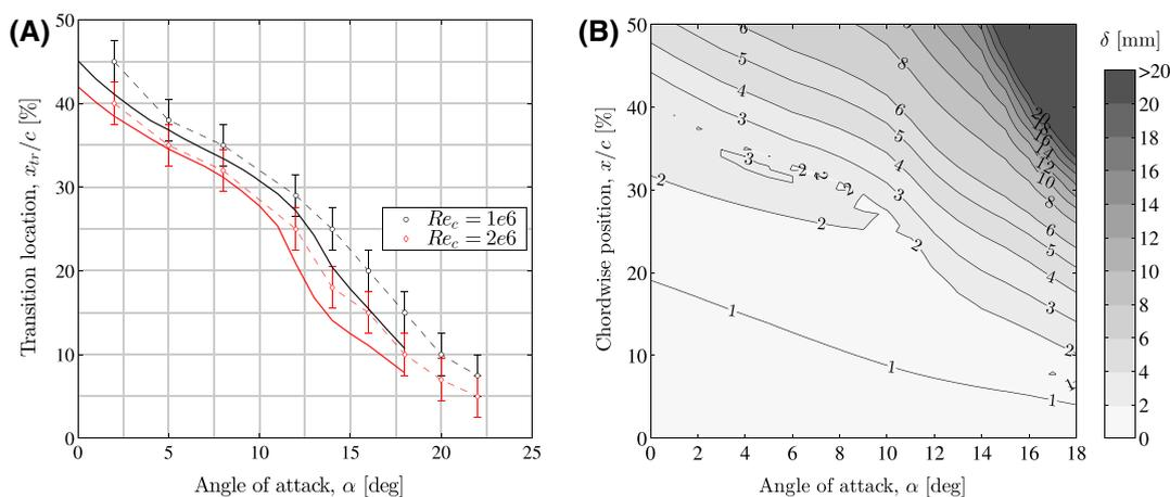
**FIGURE 6** A, Transition location on the airfoil suction side at 2 Reynolds numbers. Symbols/dashed lines indicate measurements, and solid lines represent RFOIL predictions; B, boundary layer thickness estimates in  $(\alpha, x/c)$  space at  $Re_c = 2 \times 10^6$  for natural transition [Colour figure can be viewed at [wileyonlinelibrary.com](http://wileyonlinelibrary.com)]
