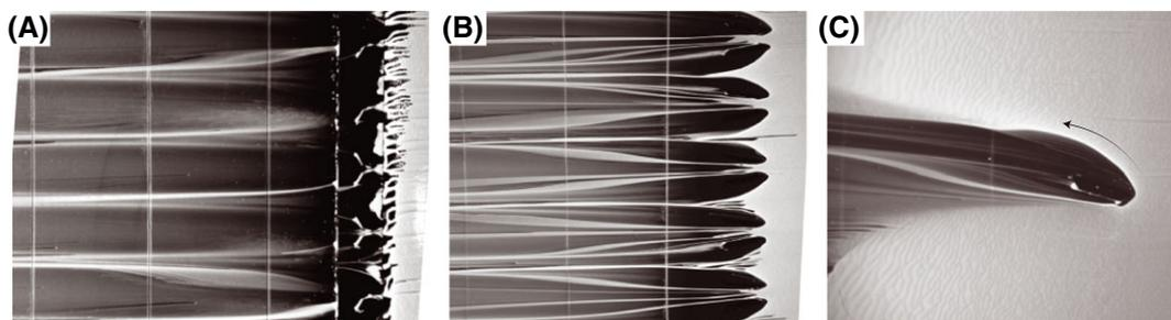
**FIGURE 12** Flow visualization of a VG array, A, with and B, without a mounting strip; C, the flow past a single vane, detailing the passage of the horseshoe vortex. Case:  $h = 10$  mm,  $x_{VG} = 20\%c$ , airfoil suction side,  $\alpha = 0^\circ$  in free transition. Flow direction: right to left [Colour figure can be viewed at [wileyonlinelibrary.com](http://wileyonlinelibrary.com)]
