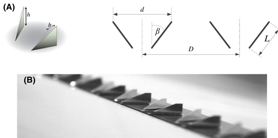
**FIGURE 1** A, Isometric view (left) and planar (right) schematic of the periodic vortex generator–array arrangement. B, Mounted cropped-delta vortex generators. Nomenclature:  $h$ , vane height;  $b$ , cropped edge length;  $d$ , intravane spacing;  $D$ , intervane spacing;  $\beta$ , geometric vane inflow angle;  $L$ , vane length [Colour figure can be viewed at [wileyonlinelibrary.com](http://wileyonlinelibrary.com)]
