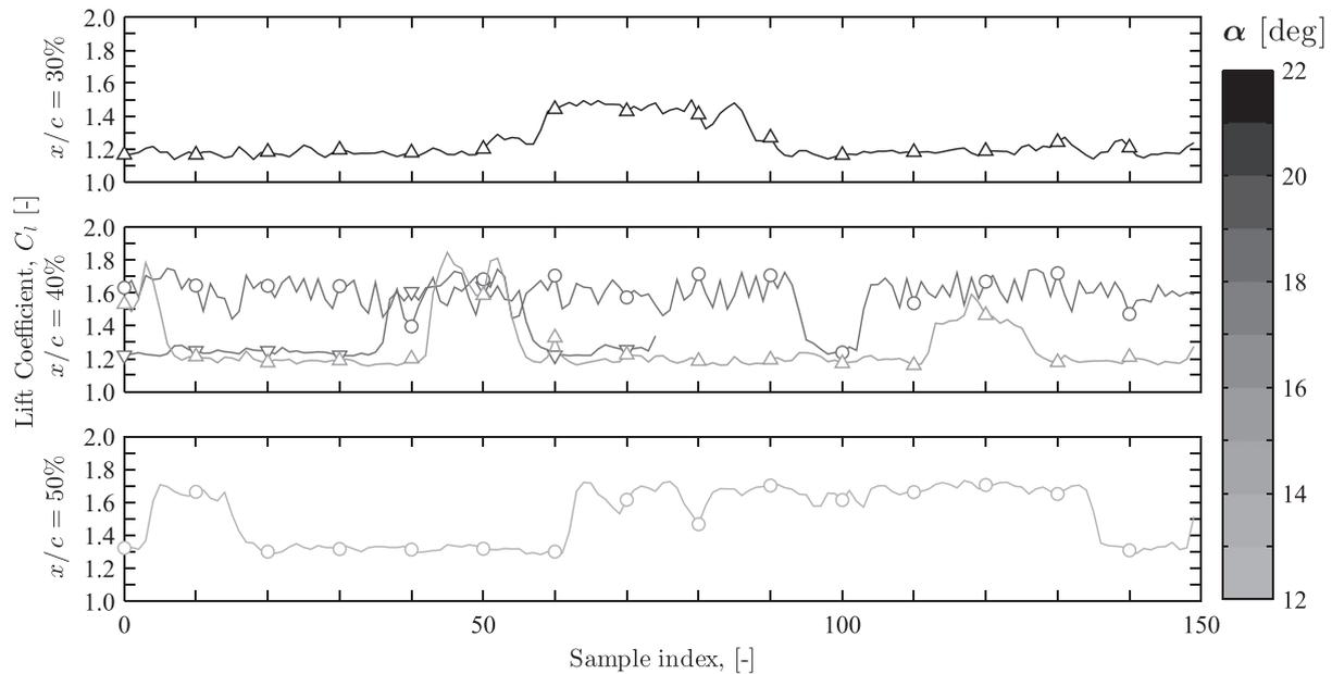
**FIGURE 19** Lift signatures exhibiting bimodal behaviour for different vortex generator heights and chordwise positions, observed at different angles of attack. Symbols:  $h = 2.5$  mm ( $\nabla$ );  $h = 5$  mm ( $\circ$ );  $h = 10$  mm ( $\Delta$ )
