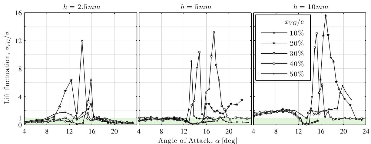
**FIGURE 20** Lift fluctuation for controlled cases relative to the uncontrolled case. Data falling outside the shaded region indicates stronger fluctuations with vortex generators [Colour figure can be viewed at [wileyonlinelibrary.com](http://wileyonlinelibrary.com)]
