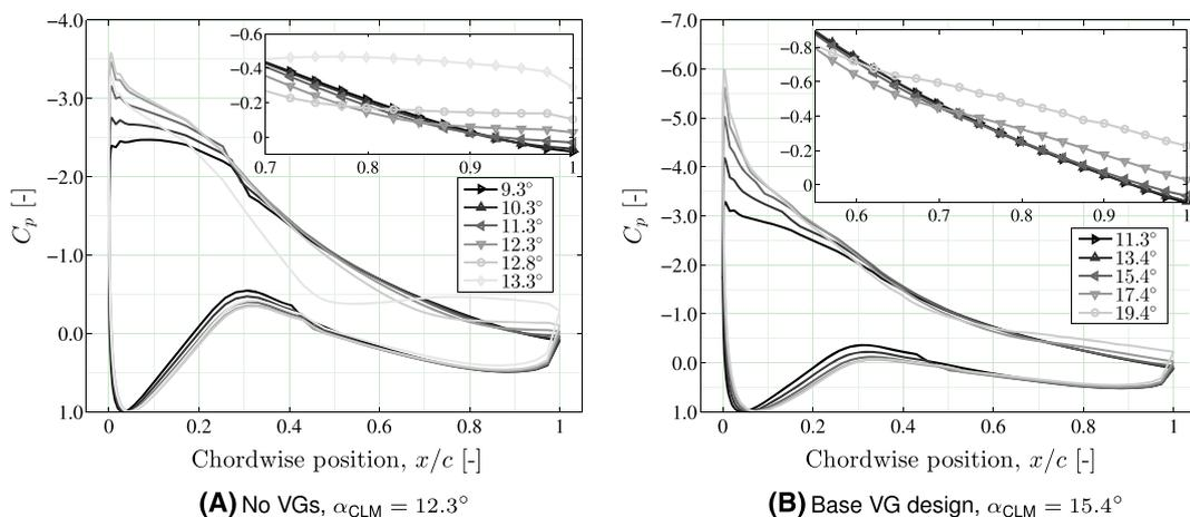
**FIGURE 17** Pressure distribution for the airfoil in free transition with and without vortex generators (VGs). Complete distributions for angles of attack around maximum lift are illustrated together with suction side pressure details for the aft portions. NoVG, uncontrolled airfoil [Colour figure can be viewed at [wileyonlinelibrary.com](http://wileyonlinelibrary.com)]
