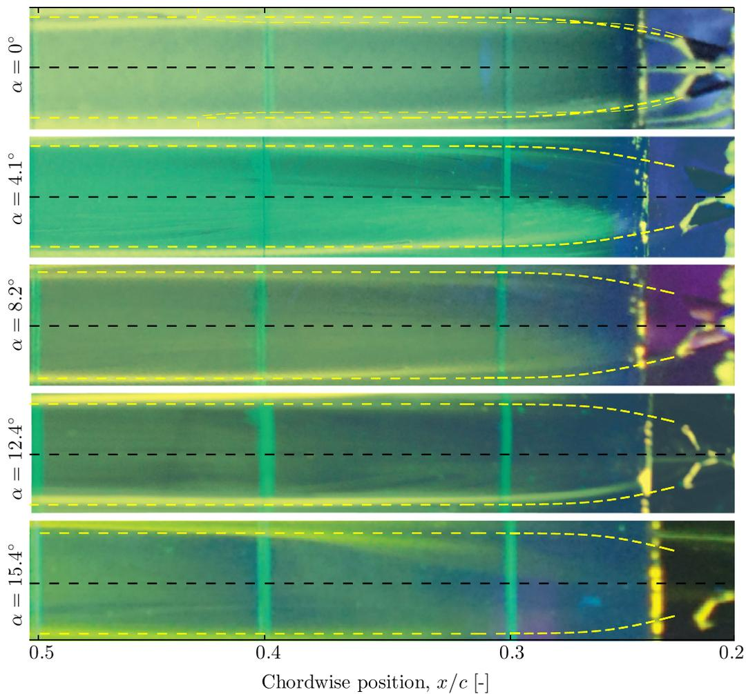
**FIGURE 10** Base design near wake oil-flow visualisations for increasing angles of attack. Flow direction: right to left [Colour figure can be viewed at [wileyonlinelibrary.com](http://wileyonlinelibrary.com)]
