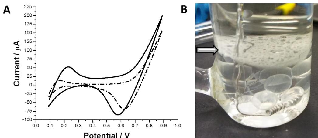
**Figure 3. A** – 1<sup>st</sup> (dash-dot line) and 50<sup>th</sup> (solid line) cycle recorded at the ITIES composed from: the aqueous phase 4  $\mu\text{M}$  Hb, pH = 2.84; the organic phase: 30% TEOS in 1,2-DCE. **B** – Photograph of the protein in silica deposit (marked with an arrow) recorded after 50 voltammetric cycles.
