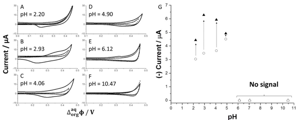
**Figure 2.** A – F solid line correspond to 8<sup>th</sup> cycle for [AP] = at indicated pH, dotted line is the blank. G – Is the peak current recorded for the reverse scan. Empty circles correspond to 1<sup>st</sup> whereas black triangles correspond to 8<sup>th</sup> cycles.
