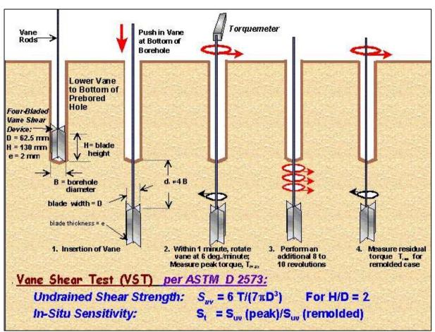
Figure 2-38: The vane shear test (English.geocpt.es).
