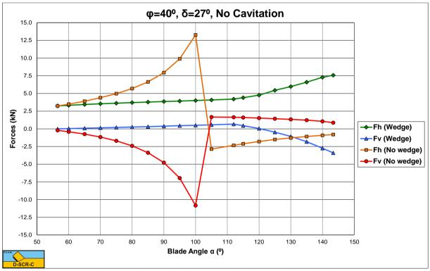
Figure P-6: No cavitation, the cutting forces as a function of the blade angle  $\alpha$  for  $\varphi$ =40° and  $\delta$ =27°.
