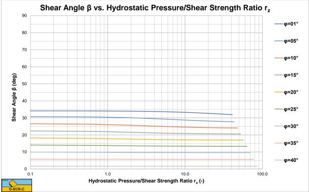
Figure 9-25: The shear angle  $\beta$  for a 110 degree blade.
