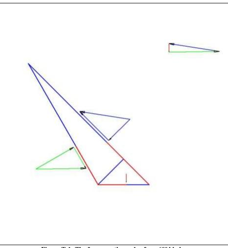
Figure T-1: The forces on the wedge for a 60° blade.
