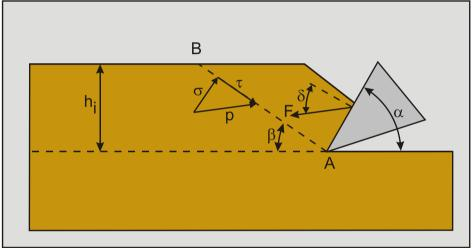
Figure 8-24: Model for shear failure by Nishimatsu (1972).
