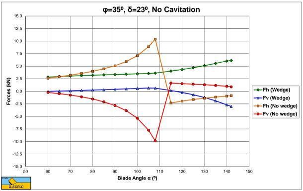
Figure P-4: No cavitation, the cutting forces as a function of the blade angle  $\alpha$  for  $\varphi$ =35° and  $\delta$ =23°.
