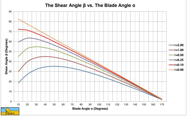
Figure V-1: The shear angle  $\beta$  as a function of the blade angle  $\alpha$  and the ac ratio r.
