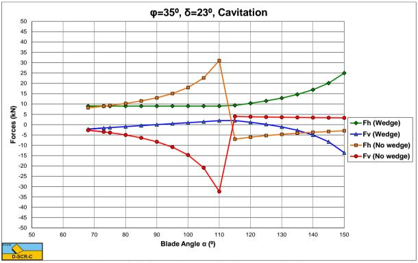
Figure Q-4: Cavitating, the cutting forces as a function of the blade angle  $\alpha$  for  $\varphi$ =35° and  $\delta$ =23°.
