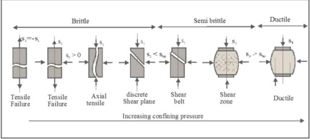
Figure 2-28: Brittle failure types (Vlasblom (2003-2007)).
