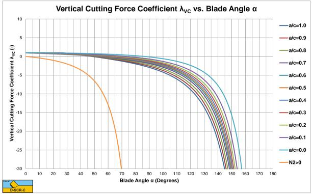
Figure V-15: The vertical cutting force coefficient  $\lambda vc$ .
