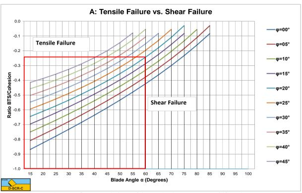
The Transition Brittle Shear/Brittle Tensile A.
