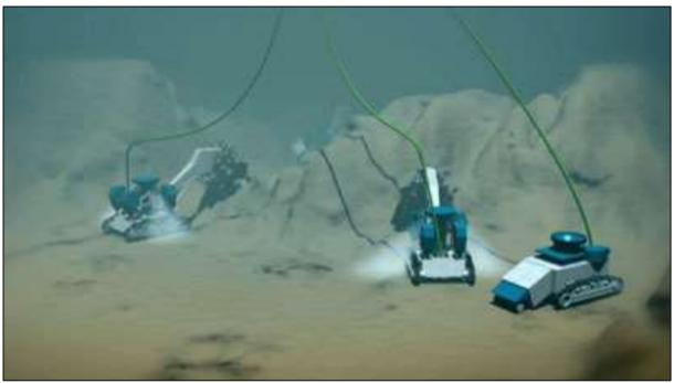
Figure Y-48: Deep sea mining excavators.
