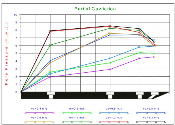
Figure 6-50: Partial cavitation limited by dissolved air,  $\alpha$ =45°, h<sub>i</sub>=7cm.
