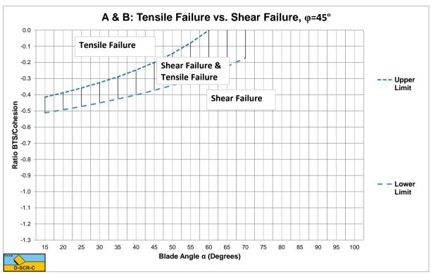
Figure W-29: The tensile/shear failure range based on BTS/Cohesion for  $\varphi$ =45°.
