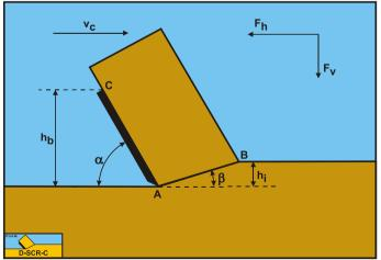
Figure 6-1: The cutting process definitions.
