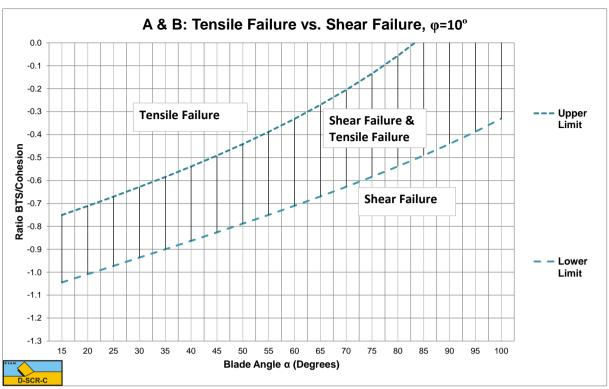
Figure W-15: The tensile/shear failure range based on BTS/Cohesion for  $\varphi$ =10°.
