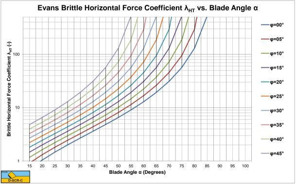
Figure 8-20: The brittle-tear horizontal force coefficient  $\lambda_{HT}$  (Evans).
