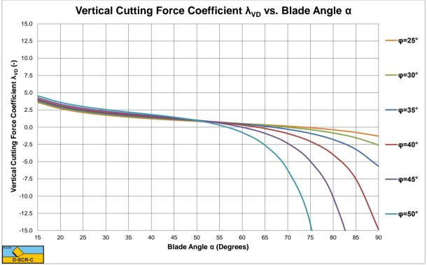
Figure B-12: The vertical cutting force coefficient  $\lambda_{VD}$  as a function of the blade angle  $\alpha$  for  $h_b/h_i=1$ .
