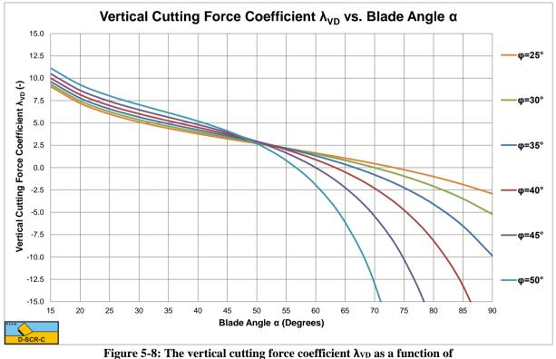
the blade angle  $\alpha$  for h<sub>b</sub>/h<sub>i</sub>=2.
