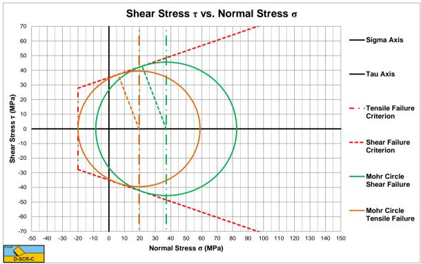
Figure 8-52: Mohr circles tensile strength -20 MPa.
