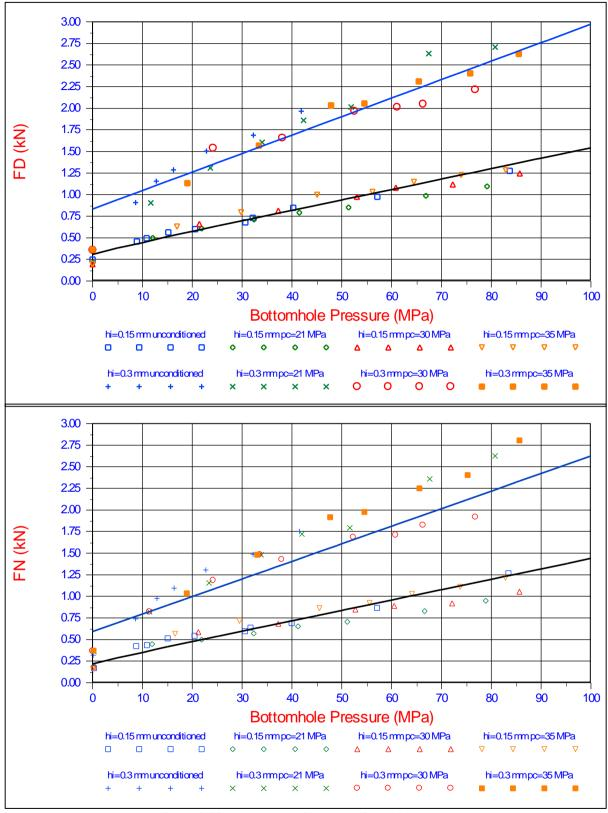
Figure 9-22: The theory of hyperbaric cutting versus the Zijsling (1987) experiments.
