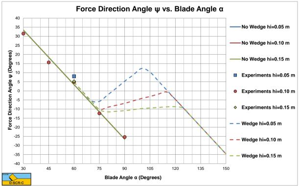
Figure 11-14: The direction of the cutting force of Hatamura & Chijiiwa (1977B) versus the calculated force direction, with and without wedge.
