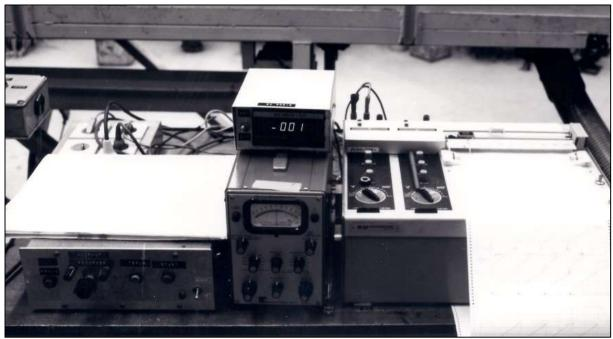
Figure 6-46: Measuring the cone resistance of the sand.
