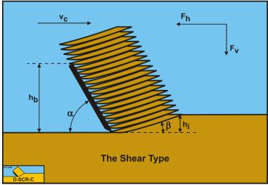
Figure 4-2: The Shear Type in saturated sand cutting.
