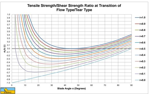
Figure 7-27: The transition Flow Type vs. Tear Type.
