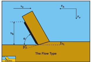
Figure 7-18: The Flow Type cutting mechanism when cutting clay.
