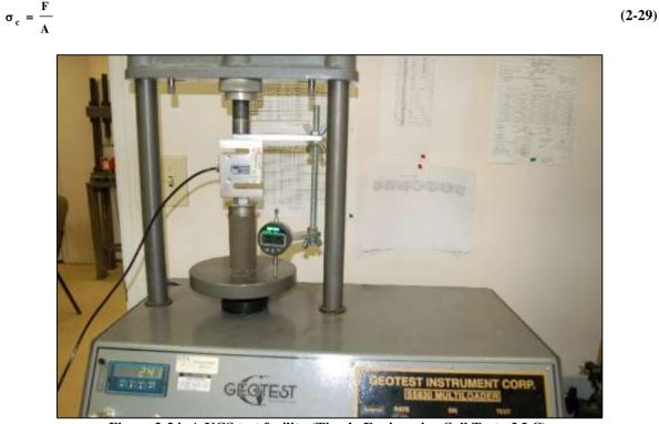
Figure 2-24: A UCS test facility (Timely Engineering Soil Tests, LLC).
