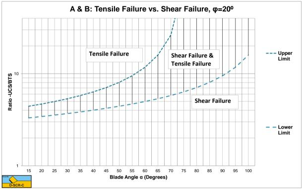
Figure W-20: The tensile/shear failure range based on UCS/BTS for  $\varphi$ =20°.
