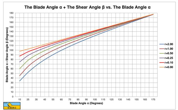
Figure 7-22: The blade angle  $\alpha$  + the shear angle  $\beta$ .
