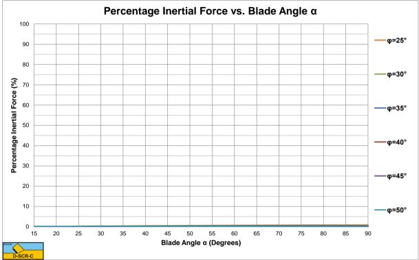
Figure 5-13: The percentage inertial force for a layer thickness  $h_i$ =1.0 m, blade height  $h_b$ =1.0 m and a cutting velocity  $v_c$ =0.5 m/sec.
