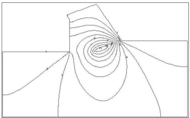
Figure 12-14: Equipotential lines of pore pressures.
