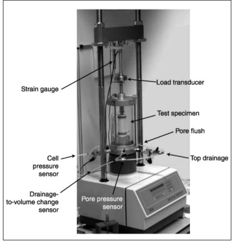
Figure 2-35: The Triaxial apparatus (www.geotechdata.info).
