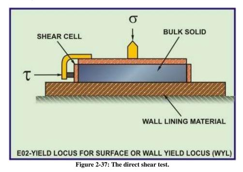
Several specimens are tested at varying confining stresses to determine the shear strength parameters, the soil cohesion (c) and the angle of internal friction (commonly friction angle) ( $\phi$ ). The results of the tests on each specimen are plotted on a graph with the peak (or residual) stress on the x-axis and the confining stress on the y-axis. The y-intercept of the curve which fits the test results is the cohesion, and the slope of the line or curve is the friction angle.
