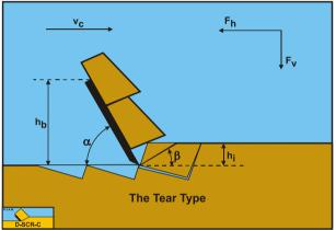
Figure 7-4: The Tear Type in clay.
