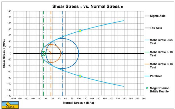
Figure 8-13: The parabolic failure criterion.
