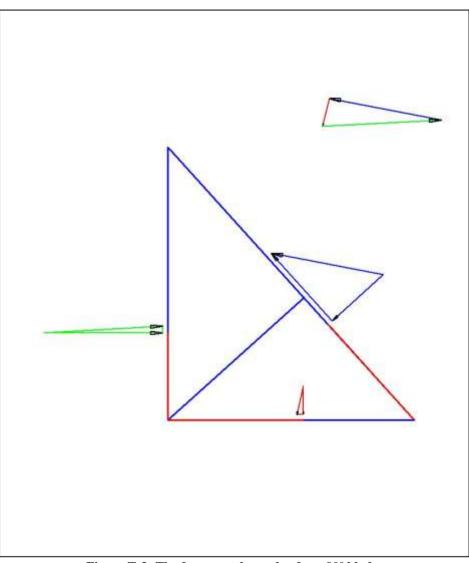
Figure T-3: The forces on the wedge for a 90° blade.
