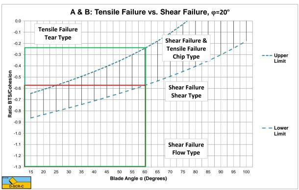
Figure W-9: The tensile/shear failure range based on BTS/Cohesion for  $\varphi$ =20°.
