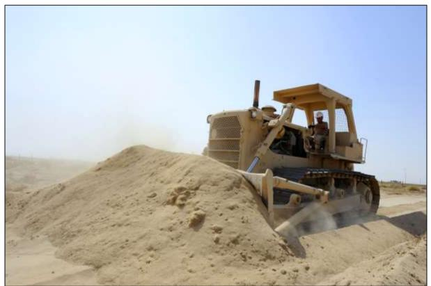
Figure 5-23: A bulldozer pushing sand (commons.wikimedia.org).
