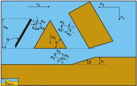
Figure 11-5: The forces on the wedge.
