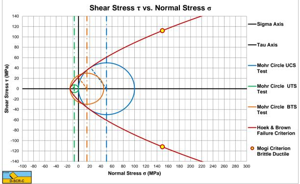
Figure 8-12: Construction Hoek & Brown failure criterion.
