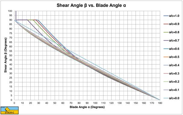
Figure V-13: The shear angle for the Curling Type
