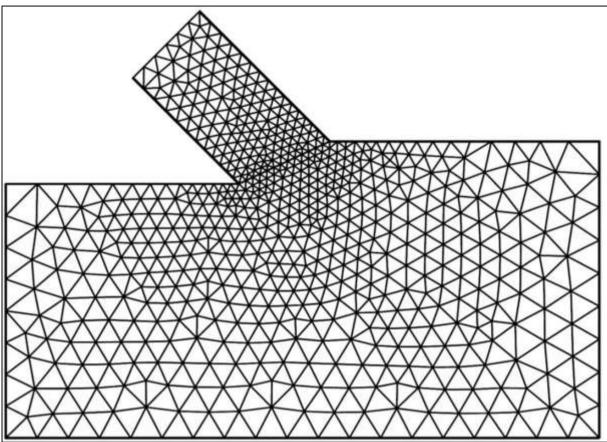
Figure 6-10: The coarse mesh as applied in the pore pressure calculations.
