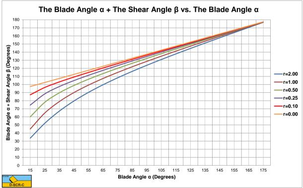
Figure V-2: The sum of the blade angle and the shear angle.
