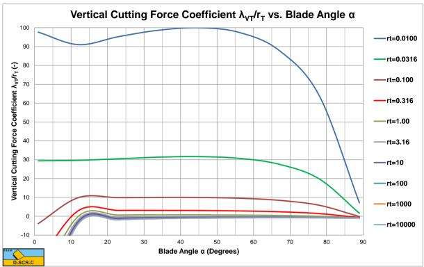
Figure 7-31: The vertical cutting force coefficient  $\lambda_{\rm VT}/r_T$ .
