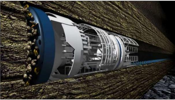
Figure Y-79: Tunnel Boring Machine (www.imaker.ca).
