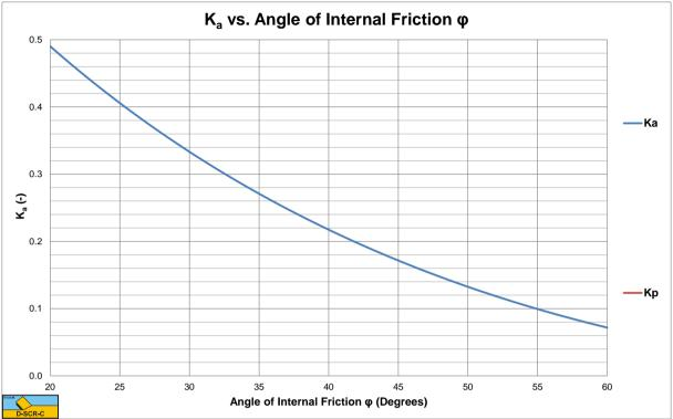
Figure 2-60: The coefficient of active soil failure Ka.
