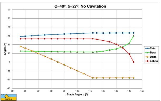
Figure P-5: No cavitation, the angles  $\theta$ ,  $\beta$ ,  $\delta_m$  and  $\lambda$  as a function of the blade angle  $\alpha$  for  $\phi$ =40° and  $\delta$ =27°.
