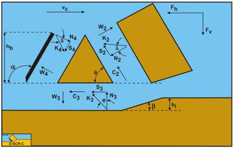
Figure 15-3: The forces on the wedge.
