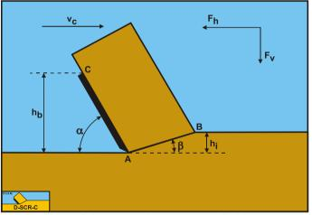
Figure 5-3: The cutting process, definitions.
