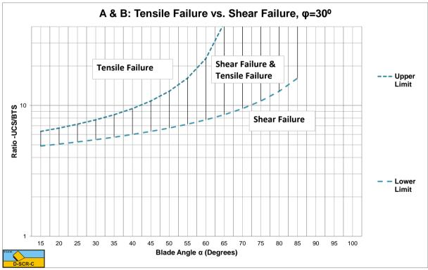
Figure W-24: The tensile/shear failure range based on UCS/BTS for  $\varphi$ =30°.
