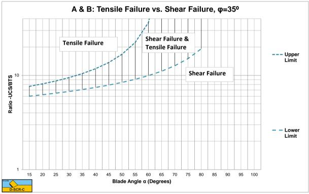
Figure W-26: The tensile/shear failure range based on UCS/BTS for  $\varphi$ =35°.
