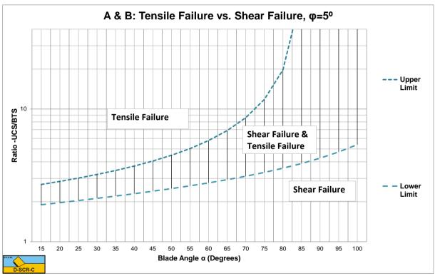
Figure W-14: The tensile/shear failure range based on UCS/BTS for  $\varphi$ =5°.
