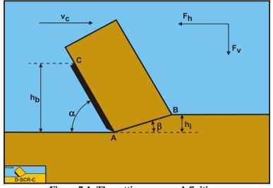
Figure 7-1: The cutting process, definitions.
