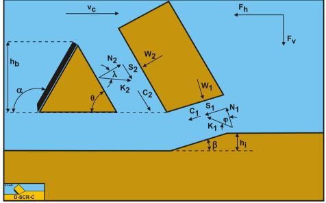
Figure 15-2: The forces on the layer cut when a wedge is present.
