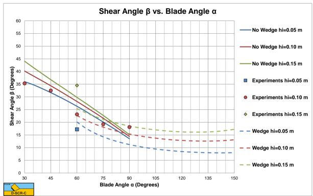
Figure 11-11: The shear angle of Hatamura & Chijiiwa (1977B) versus the calculated shear angles, with and without wedge.
