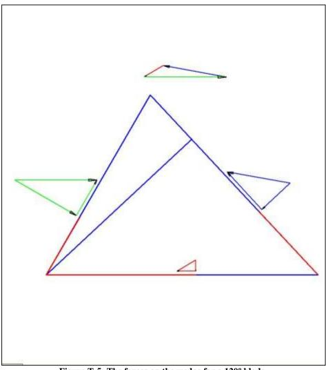
Figure T-5: The forces on the wedge for a 120° blade.
