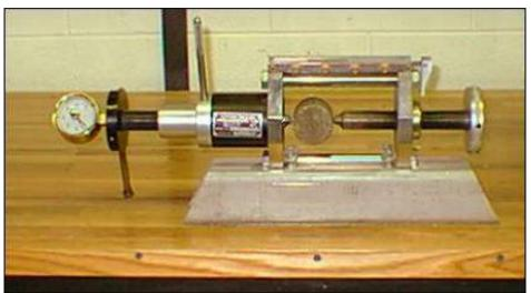
Figure 2-40: Point load test facility (inside.mines.edu).
