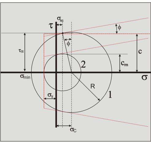
Figure 3-13: The Mohr circles of the Tear Type.
