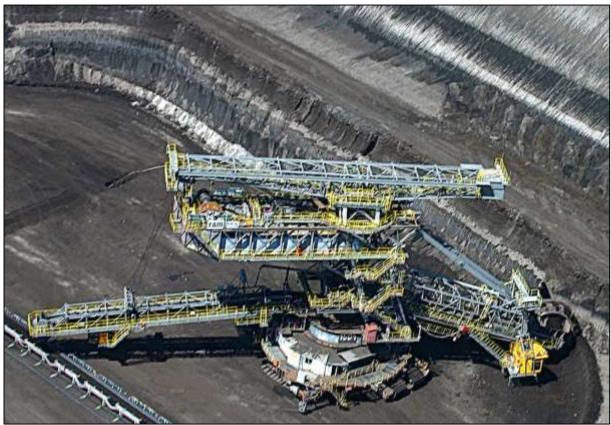
Figure Y-43: A bucket wheel excavator (www.directindustry.com).
