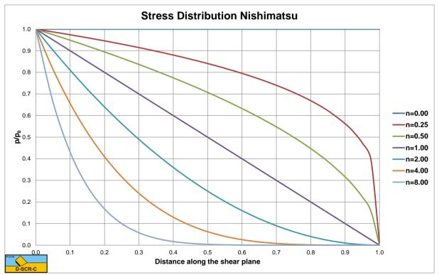
Figure 8-25: The stress distribution along the shear plane.
