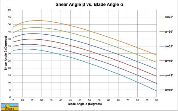
Figure B-10: The shear angle  $\beta$  as a function of the blade angle  $\alpha$  for  $h_b/h_i{=}1.$
