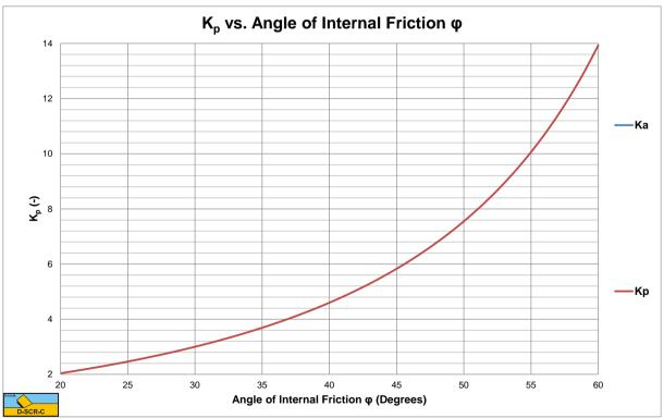
Figure 2-61: The coefficient of passive soil failure K<sub>p</sub>.
