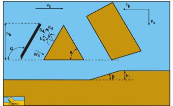
Figure 12-6: The forces on the blade in saturated sand with a wedge.
