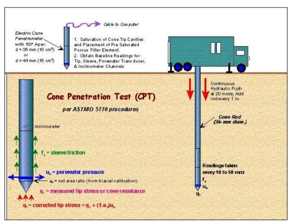
Figure 2-32: A typical CPT test setup (www.geotechdata.com).
