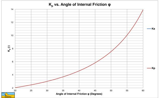
Figure A-3: The coefficient of passive soil failure K<sub>p</sub>.
