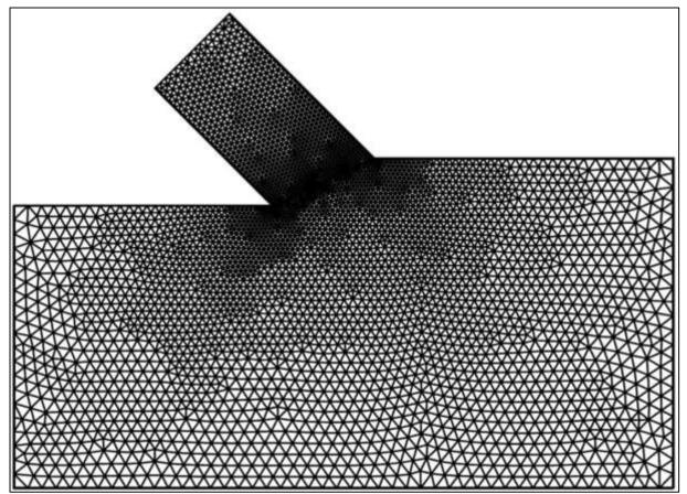
Figure 6-11: The fine mesh as applied in the pore pressure calculations.
