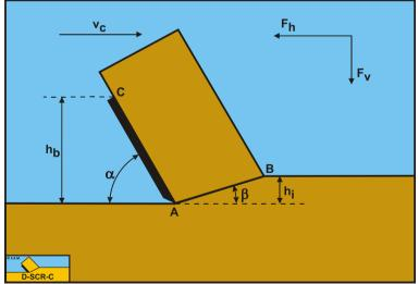
Figure 3-2: The cutting process, definitions.
