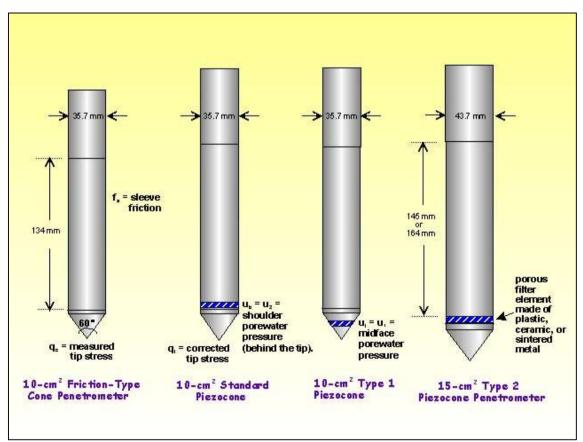
Figure 2-33: Several configurations of cones (www.geotechdata.info).
