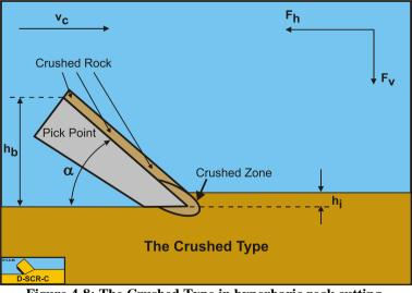
Figure 4-8: The Crushed Type in hyperbaric rock cutting.
