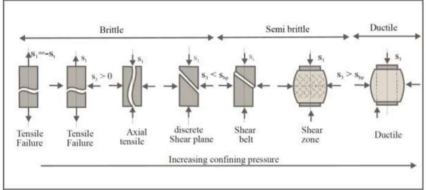
Figure 8-8: Brittle, semi brittle and ductile failure.
