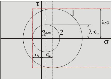
Figure 7-28: The Mohr circles when cutting clay.
