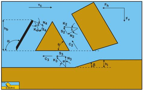
Figure 14-3: The forces on the wedge.
