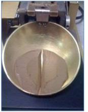
Figure 2-19: Liquid limit device.
