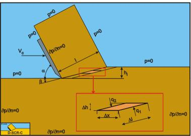
Figure 6-8: The volume balance over the shear zone.
