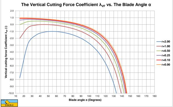
Figure 7-24: The vertical cutting force coefficient  $\lambda_{VF}$  as a function of the blade angle and the ac ratio r.
