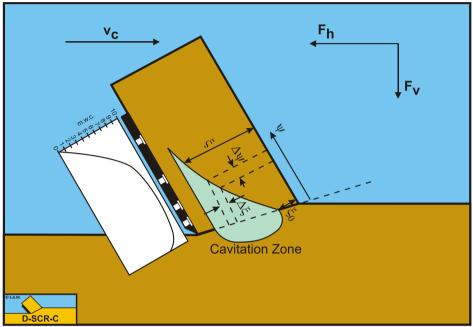
Figure 6-49: The development of cavitation over the blade.
