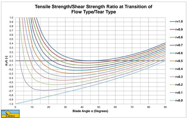
Figure V-7: The transition Flow Type vs. Tear Type.
