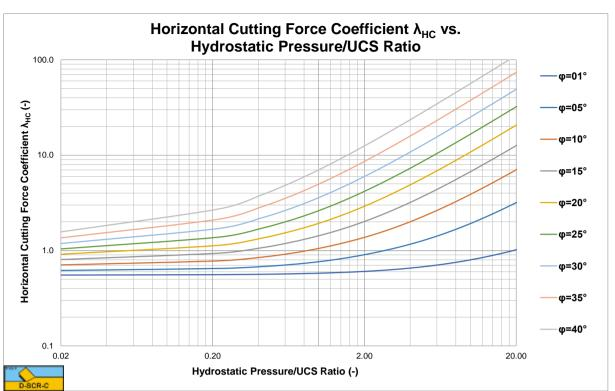
Figure X-3: The horizontal cutting force coefficient  $\lambda_{\rm HC}$  for a 30 degree blade.
