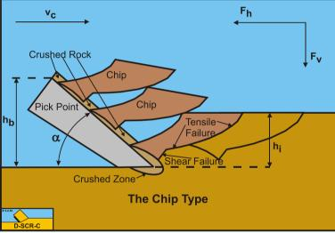
Figure 4-7: The Chip Type in atmospheric rock cutting.
