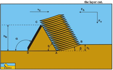
Figure 11-3: The cutting mechanism.
