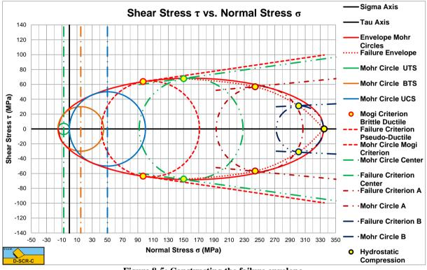
Figure 8-5: Constructing the failure envelope.
