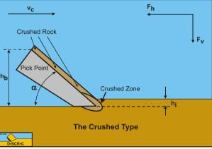
Figure 3-5: The Crushed Type.
