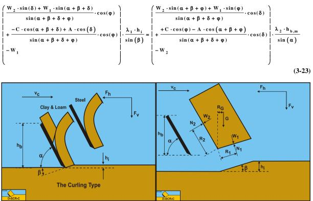
Figure 3-8: The Curling Type of cutting mechanism. Figure 3-9: The general equilibrium of moments.
