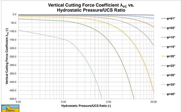
Figure X-34: The vertical cutting force coefficient  $\lambda_{VC}$  for a 120 degree blade.
