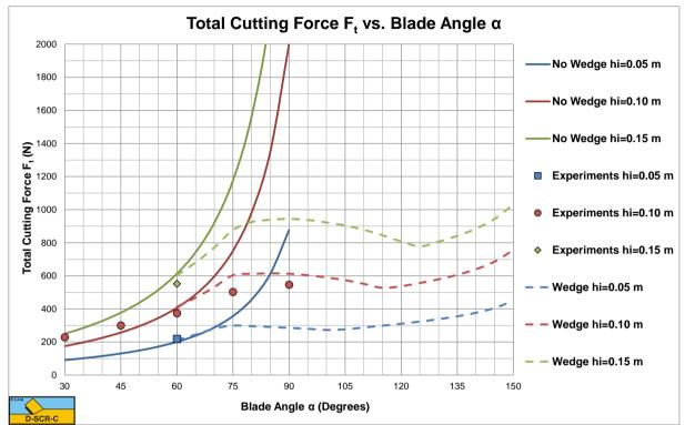
Figure 11-13: The total force of Hatamura & Chijiiwa (1977B) versus the calculated total force, with and without wedge.
