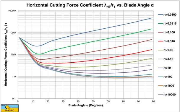
Figure 7-30: The horizontal cutting force coefficient  $\lambda_{\text{HT}}/r_{\text{T}}$ .
