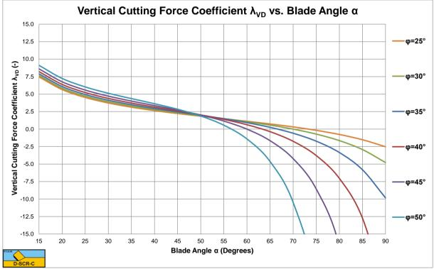
Figure B-15: The vertical cutting force coefficient  $\lambda_{VD}$  as a function of the blade angle  $\alpha$  for  $h_b/h_i=2$ .
