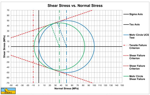
Figure 16-10: The Mohr circles with tensile strength of -10 MPa (UCS=100 MPa,  $\varphi$ =20°). Shear Failure.
