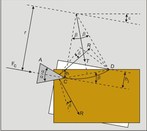
Figure 8-22: The model of Evans under an angle ε.
