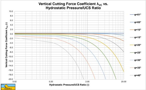
Figure X-19: The vertical cutting force coefficient  $\lambda_{\rm VC}$  for a 75 degree blade.
