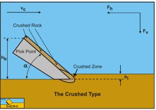
Figure 9-6: The Crushed Type cutting mechanism.
