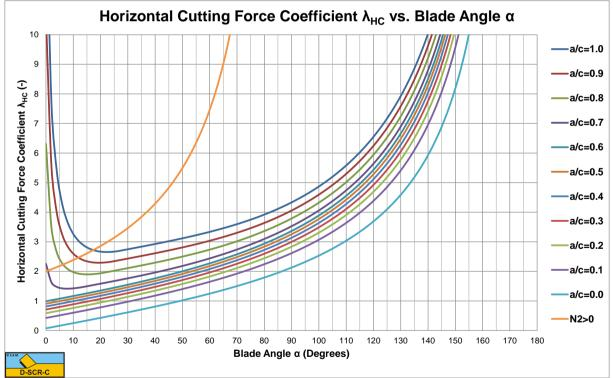
Figure 7-36: The horizontal cutting force coefficient  $\lambda_{\rm HC}$ .
