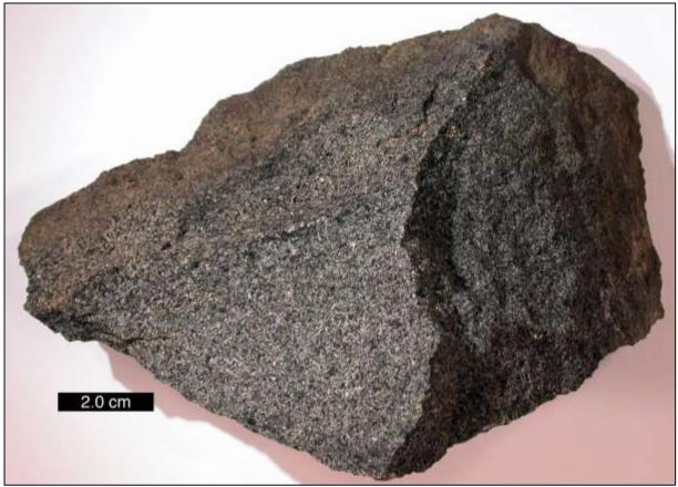
Figure 2-11: Sample of igneous gabbro, Rock Creek Canyon, California (source Wikimedia).
