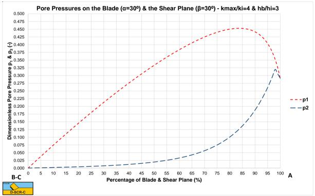
Figure 6-22: The dimensionless pressures on the blade and the shear plane,  $\alpha$ =30°,  $\beta$ =30°,  $k_i/k_{max}$ =0.25,  $h_i/h_b$ =1/3.
