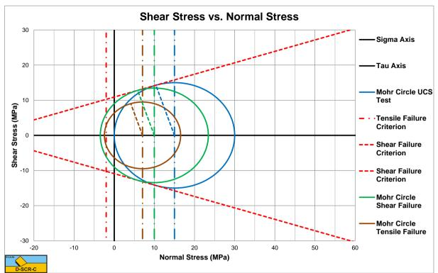
Figure 16-8: The Mohr circles for a tensile strength of -2 MPa. Tensile Failure.
