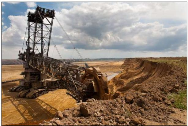
Figure Y-44: Giant bucket wheel excavator.
