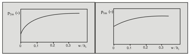
Figure 6-18: The water pore pressures on the blade as function of the length of the wear section w. Figure 6-19: The water pore pressure in the shear zone as function of the length of the wear section w.
