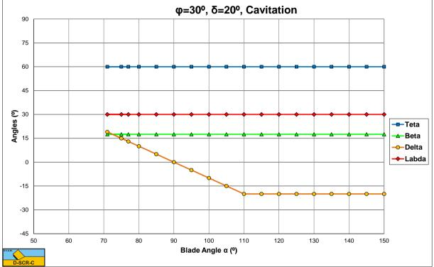
Figure 12-24: Cavitating, the angles  $\theta$ ,  $\beta$ ,  $\delta_m$  and  $\lambda$  as a function of the blade angle  $\alpha$  for  $\phi=30^{\circ}$  and  $\delta=20^{\circ}$ .
