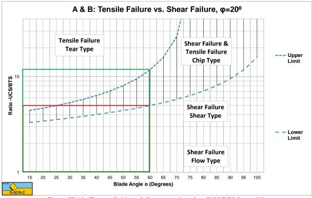
Figure W-10: The tensile/shear failure range based on UCS/BTS for  $\varphi$ =20°.
