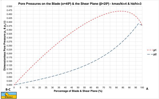
Figure 6-23: The dimensionless pressures on the blade and the shear plane,  $\alpha$ =45°,  $\beta$ =25°, k<sub>i</sub>/k<sub>max</sub>=0.25, h<sub>i</sub>/h<sub>b</sub>=1/2.
