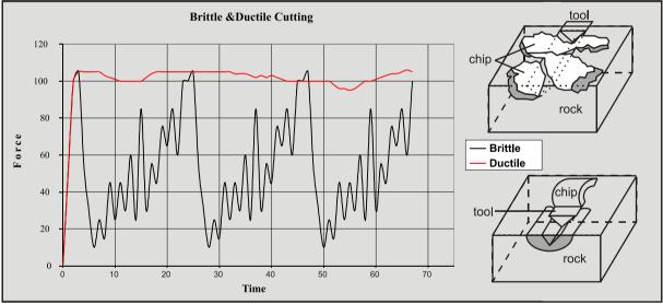
Figure 8-1: Ductile and brittle cutting Verhoef (1997).
