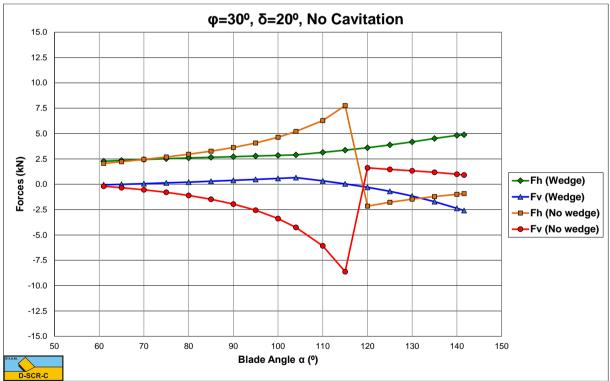
Figure 12-23: No cavitation, the cutting forces as a function of the blade angle  $\alpha$  for  $\varphi$ =30° and  $\delta$ =20°.
