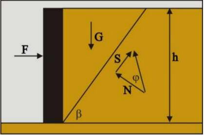
Figure 2-51: Active soil failure.
