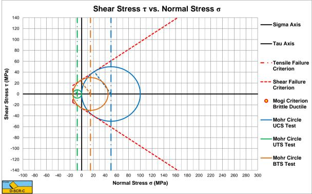
Figure 8-10: Construction of the angle of internal friction BTS-UCS based.
