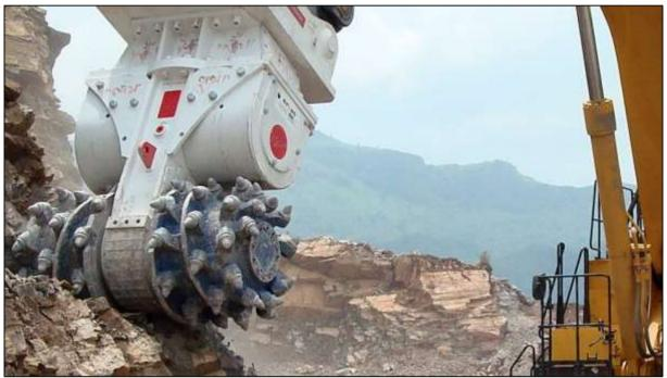
Figure Y-72: Double head drum cutter (www.drumcutters.com).
