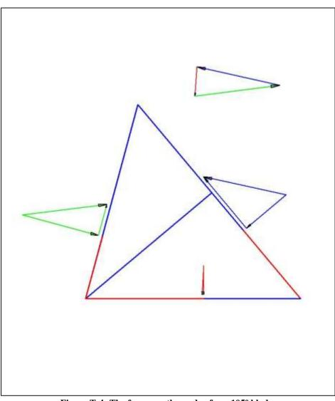
Figure T-4: The forces on the wedge for a 105° blade.
