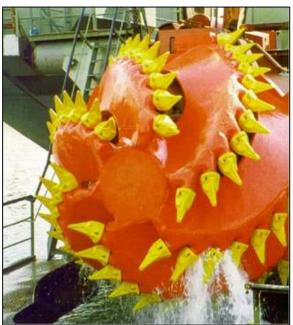
Figure Y-13: A rock cutter head.
