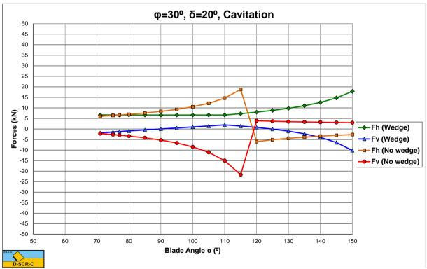
Figure 12-25: Cavitating, the cutting forces as a function of the blade angle  $\alpha$  for  $\varphi$ =30° and  $\delta$ =20°.
