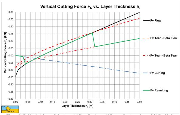
Figure 7-40: Vertical force; Cohesion c=1 kPa, adhesion a=1 kPa, tensile strength  $\sigma_T$ =-0.3 kPa, blade height h<sub>b</sub>=0.1 m, blade angle  $\alpha$ =55°
