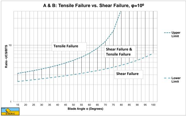
Figure W-16: The tensile/shear failure range based on UCS/BTS for  $\varphi$ =10°.
