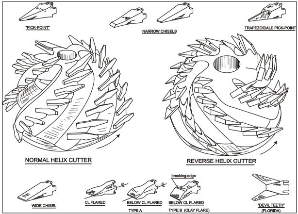
Figure 1-2: A rock cutter head with pick points.
