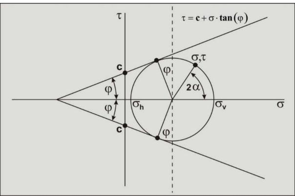
Figure 2-48: The Mohr circle for soil with cohesion.
