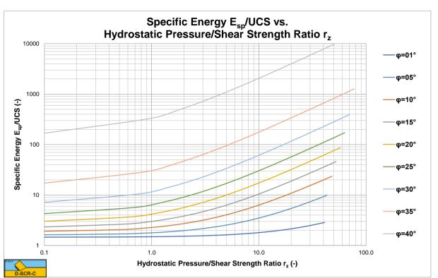
Figure 9-28: The E<sub>sp</sub>/UCS ratio, for a 110 degree blade.
