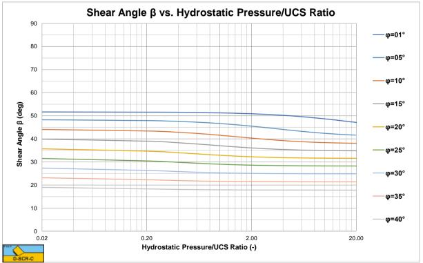
Figure X-17: The shear angle  $\beta$  for a 75 degree blade.
