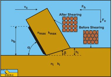
Figure 6-7: The cutting process modeled as a continuous process.
