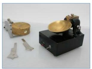
Figure 2-20: Liquid limit device.
