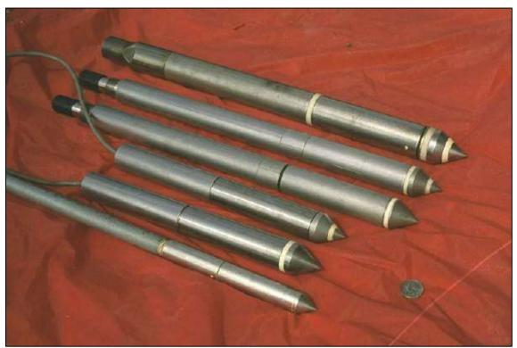
Figure 2-34: Several cone configurations.
