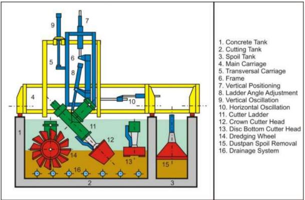
Figure 12-29: Cross section of the cutting tank.
