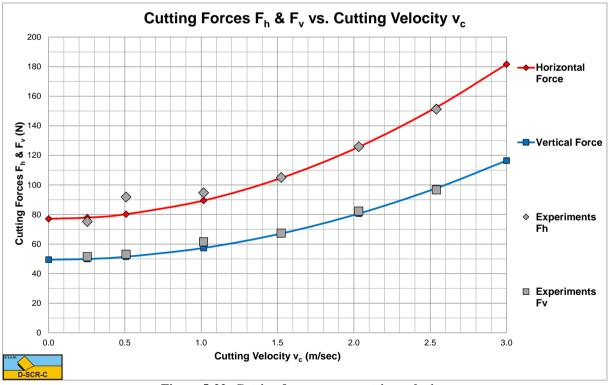
Figure 5-22: Cutting forces versus cutting velocity.
