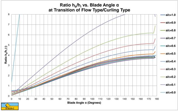
Figure 7-38: The ratio h<sub>b</sub>/h<sub>i</sub> at the transition Flow Type/Curling Type.
