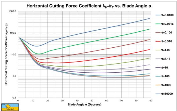
Figure V-9: The horizontal cutting force coefficient  $\lambda_{\text{HT}}/r_{\text{T}}$ .
