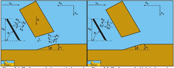
Figure 5-4: The forces on the layer cut in dry sand. Figure 5-5: The forces on the blade in dry sand.
