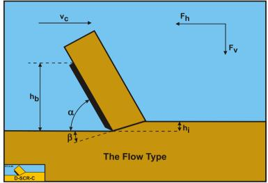
Figure 8-27: The Flow Type cutting mechanism in ductile rock cutting.
