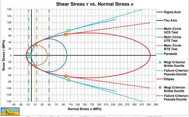
Figure 8-14: The Parabolic and Ellipsoid failure envelopes, with a=1.75·UCS.
