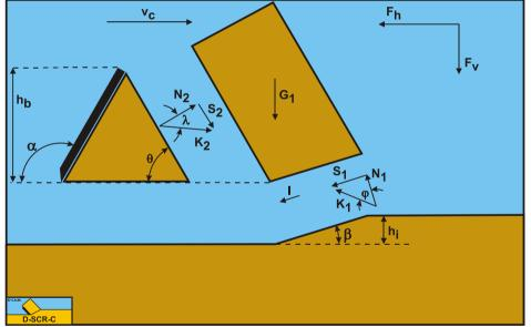
Figure 11-4: The forces on the layer cut when a wedge is present.
