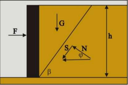
Figure 2-54: Passive soil failure.
