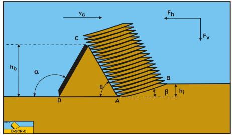
Figure 12-3: The cutting mechanism.
