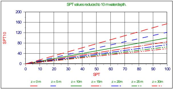
Figure 6-30: SPT values reduced to 10m water depth.
