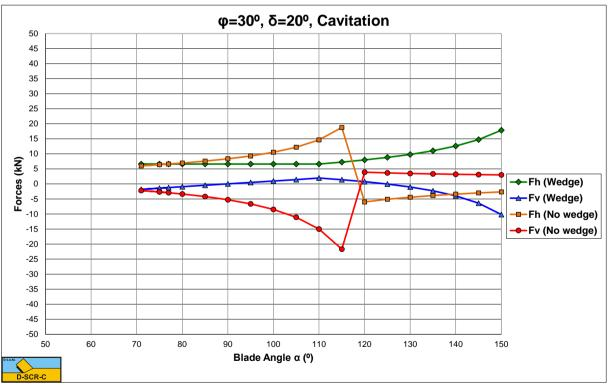
Figure Q-2: Cavitating, the cutting forces as a function of the blade angle  $\alpha$  for  $\varphi$ =30° and  $\delta$ =20°.
