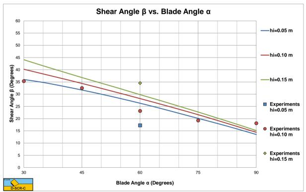
Figure 5-19: The shear angle versus the blade angle.
