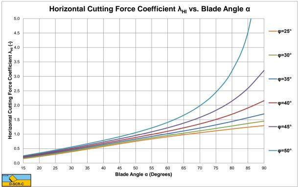
Figure 5-16: The horizontal cutting force coefficient  $\lambda_{\rm HI}$ .
