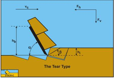
Figure 7-26: The Tear Type cutting mechanism in clay.
