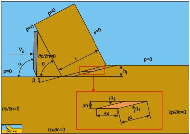
Figure 12-7: The volume balance over the shear zone.
