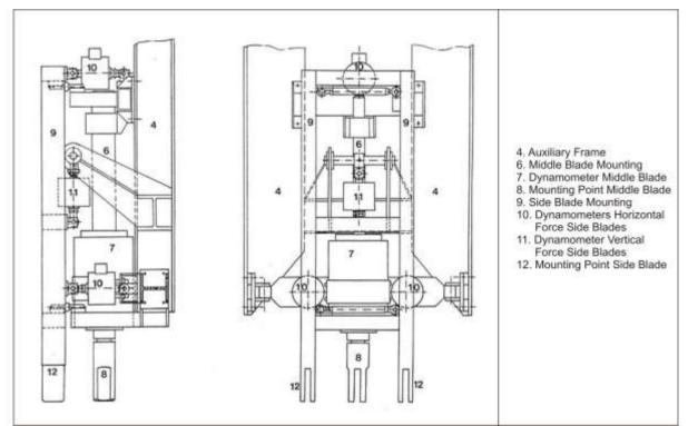
Figure 6-41: The construction in which the blades are mounted.
