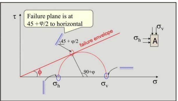
Figure 2-52: The Mohr circle for active soil failure.
