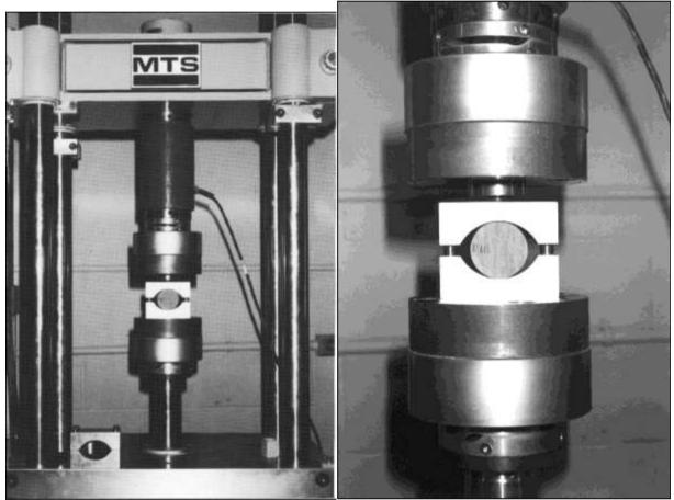
Figure 2-41: Brazilian splitting tension test.
