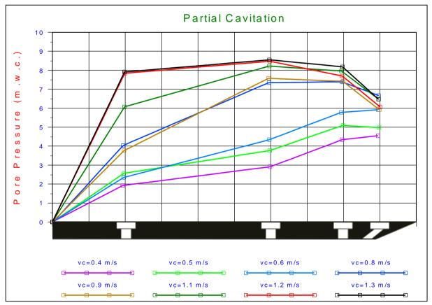
Figure M-5: Measured absolute pore pressures.
