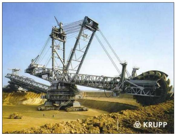
Figure Y-42: 95m high, 215m long, 45500 tons, \$100 million, 10 m/min, 76000 m<sup>3</sup>/day.
