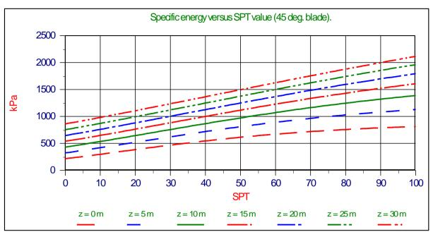
Figure 6-31: Specific energy versus SPT value (45 deg. blade).
