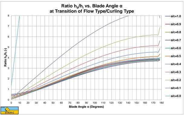
Figure V-12: The ratio h<sub>b</sub>/h<sub>i</sub> at the transition Flow Type/Curling Type.
