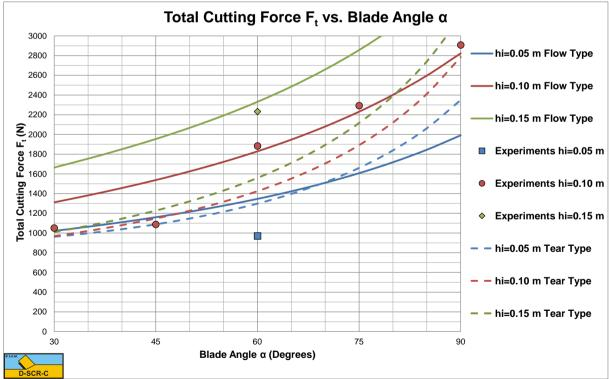
Figure 7-45: The total cutting force measured and calculated.
