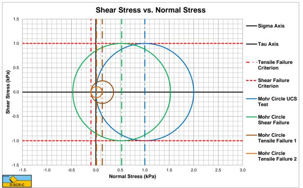
A tensile strength of -20 kPa gives a  $\sigma_T/c$  ratio of -0.1. With an **ac** ratio of r=0.05 this ratio should be below -0.5 according to Figure 7-27 (Figure 7-26, 1<sup>st</sup> edition) for the **Flow Type**, it is not, so we have the **Tear Type**.
