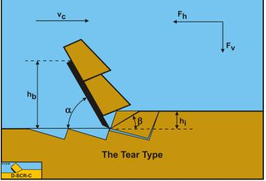
Figure 4-5: The Tear Type in clay and loam cutting.
