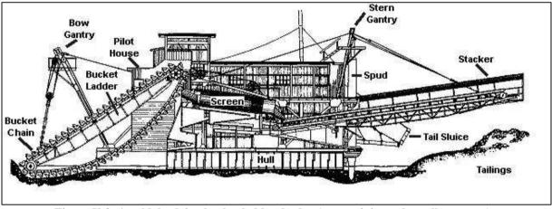
Figure Y-2: A gold dredging bucket ladder dredge (www.miningandmetallurgy.com).
