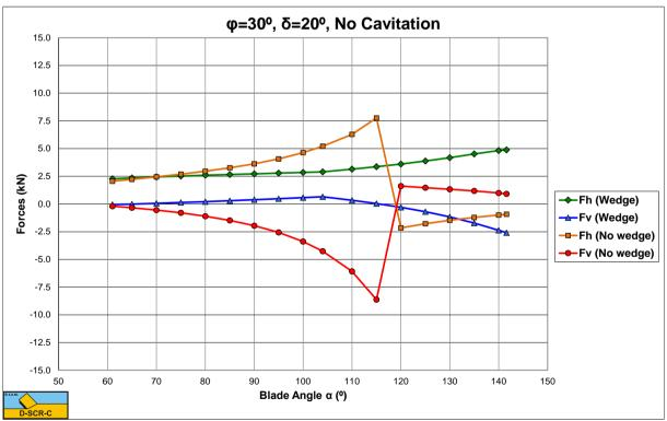
Figure P-2: No cavitation, the cutting forces as a function of the blade angle  $\alpha$  for  $\varphi$ =30° and  $\delta$ =20°.
