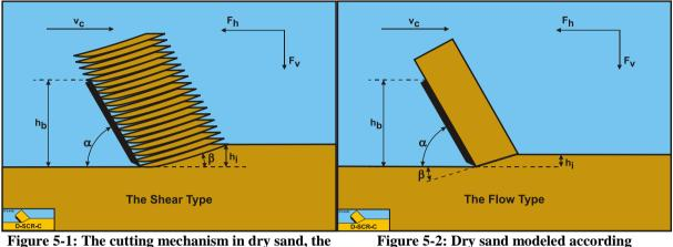
Figure 5-1: The cutting mechanism in dry sand, the Shear Type.
