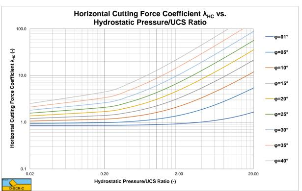
Figure X-8: The horizontal cutting force coefficient  $\lambda_{\rm HC}$  for a 45 degree blade.
