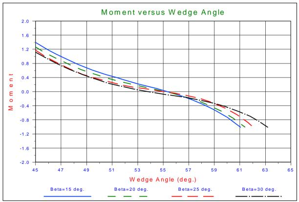
Figure 12-19: Moment versus wedge angle  $\theta$  by using polynomial regression for:  $\alpha$ =90<sup>0</sup>;  $\beta$ =15<sup>0</sup>,20<sup>0</sup>,25<sup>0</sup>,30<sup>0</sup>;  $\delta$ =28<sup>0</sup>;  $\varphi$ =42<sup>0</sup>;  $h_i$ =1;  $h_b$ =3;  $k_i/k_{max}$ =0.25
