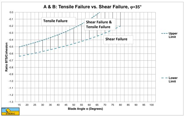
Figure W-25: The tensile/shear failure range based on BTS/Cohesion for  $\varphi$ =35°.
