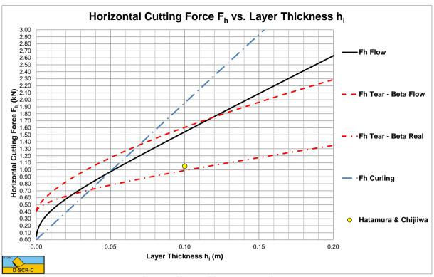
Figure 7-48: The 30 degree experiment.
