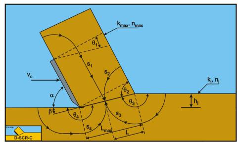
Figure 6-20: The flow lines used in the analytical method.
