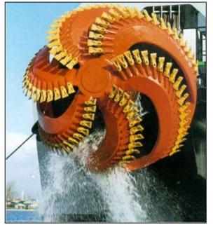
Figure Y-12: A sand cutter head.
