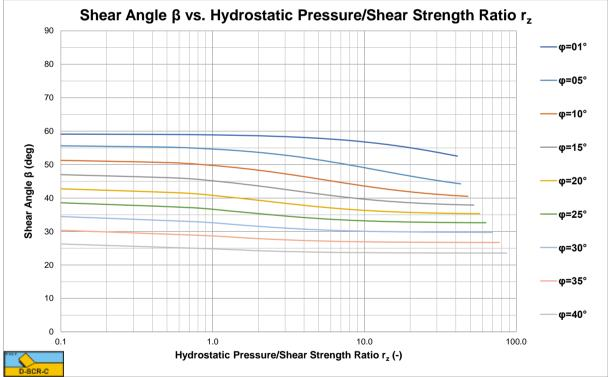
Figure 9-18:The shear angle β for a 60 degree blade
