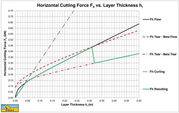
Figure 7-39: Horizontal force; cohesion c=1 kPa, adhesion a=1 kPa, tensile strength  $\sigma_T$ =-0.3 kPa, blade height  $h_b$ =0.1 m, blade angle  $\alpha$ =55°
