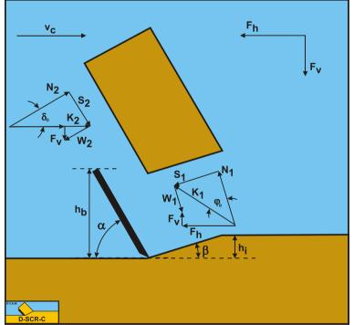
Figure 6-6: The forces on the blade when cutting water saturated sand.
