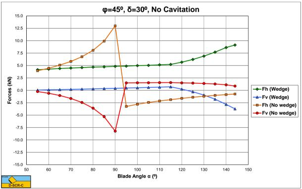
Figure P-8: No cavitation, the cutting forces as a function of the blade angle  $\alpha$  for  $\varphi$ =45° and  $\delta$ =30°.
