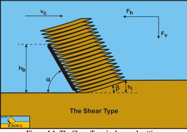
Figure 4-1: The Shear Type in dry sand cutting.
