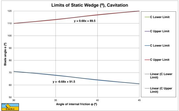
Figure 12-27: The lower and upper limit where a static wedge can exist for the cavitating cutting process.
