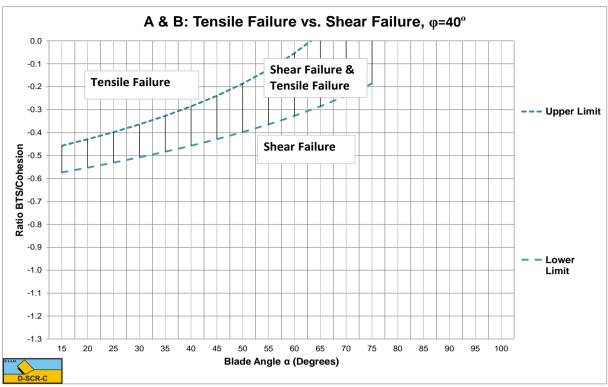
Figure W-27: The tensile/shear failure range based on BTS/Cohesion for  $\varphi$ =40°.
