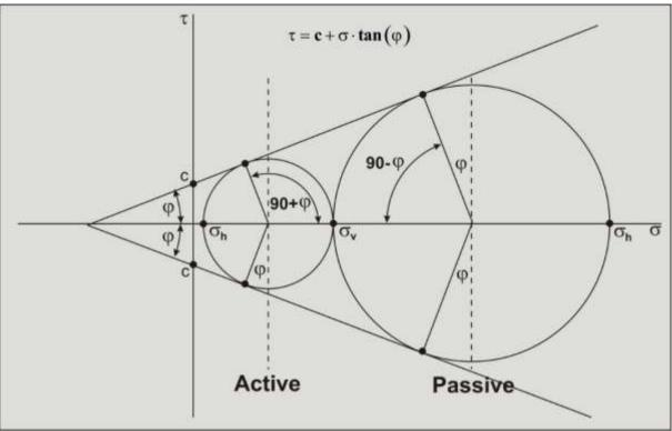
Figure 2-58 gives a summary of the Mohr circles for Active and Passive failure for a soil with cohesion.
