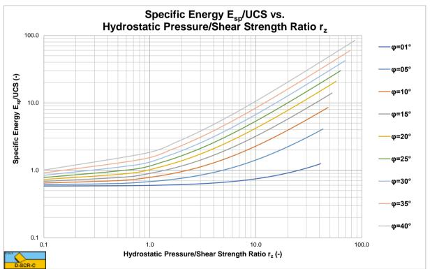
Figure 9-12: The E<sub>sp</sub>/UCS ratio, for a 60 degree blade, h<sub>b</sub>/h<sub>i</sub>=1.
