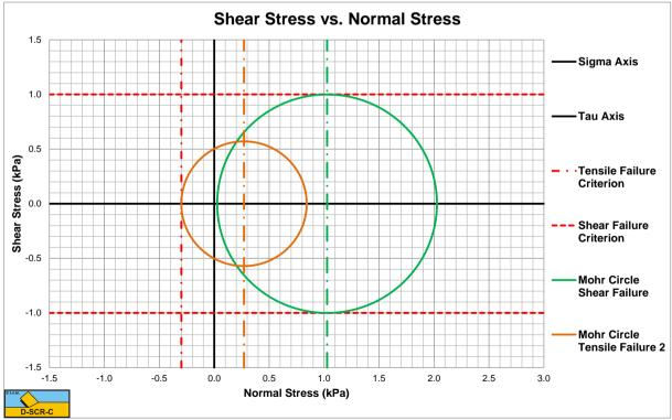
Figure 7-41: The Mohr circles for h<sub>i</sub>=0.1 m, two possibilities.
