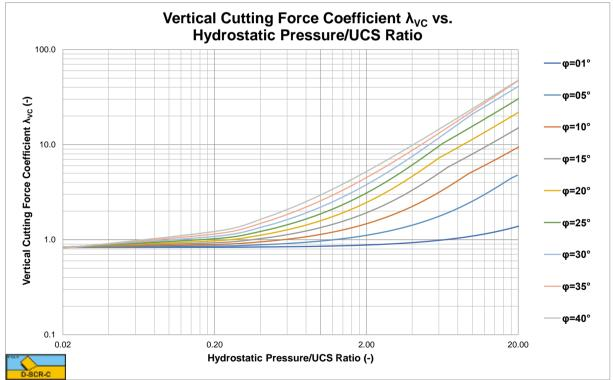
Figure X-9: The vertical cutting force coefficient  $\lambda_{\rm VC}$  for a 60 degree blade.
