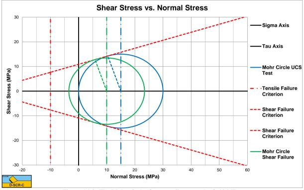
Figure 16-9: The Mohr circles for a tensile strength of -10 MPa. Shear Failure.
