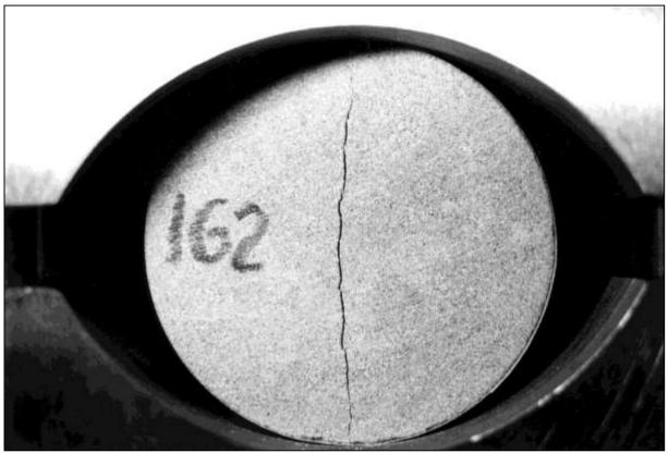
Figure 2-43: A BTS test after failure.
