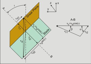
Figure 3-17: Velocity conditions.
