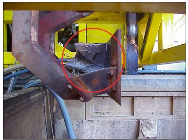
Figure 12-33: Cover with camera behind the blade.
