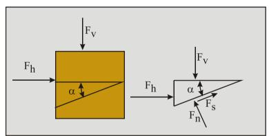
Figure 2-45: The forces on a soil element.
