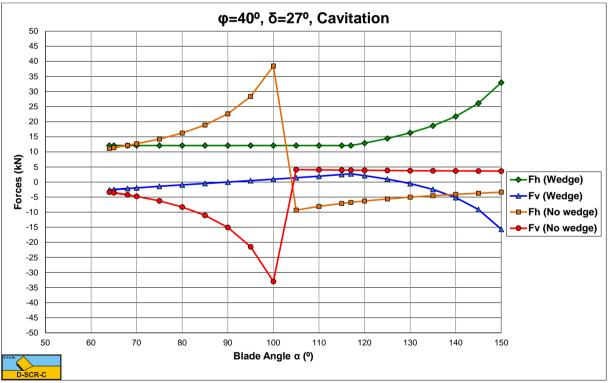
Figure Q-6: Cavitating, the cutting forces as a function of the blade angle  $\alpha$  for  $\varphi$ =40° and  $\delta$ =27°.
