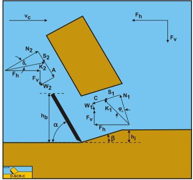
Figure 3-14: The forces on the layer cut.
