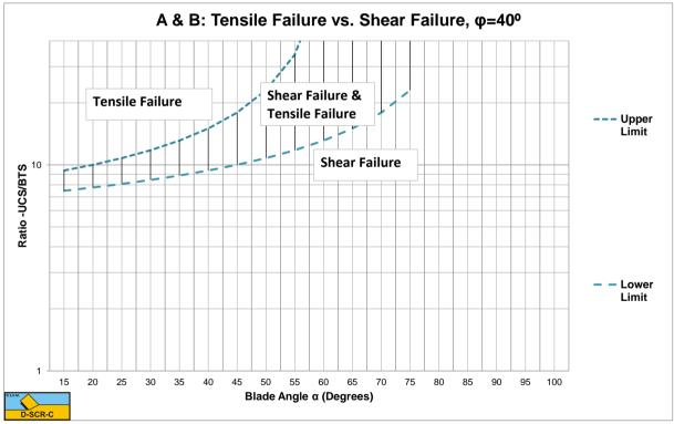
Figure W-28: The tensile/shear failure range based on UCS/BTS for  $\varphi$ =40°.
