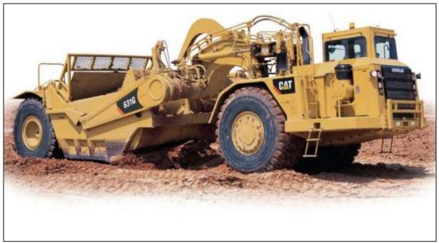
Figure Y-70: Caterpillar 631G tractor scraper.
