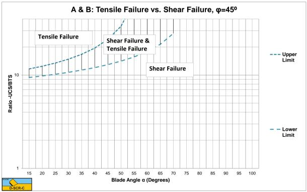
Figure W-30: The tensile/shear failure range based on UCS/BTS for  $\varphi$ =45°.
