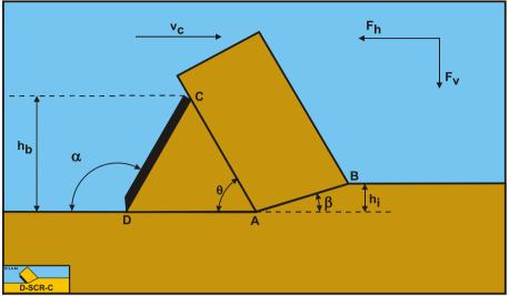
Figure 12-2: Sand cutting with a wedge, definitions.
