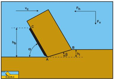
Figure 8-26: The definitions of the cutting process.
