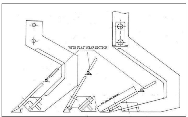
Figure 6-45: The center blade of 30°, 45° and 60°, with and without wear flat.
