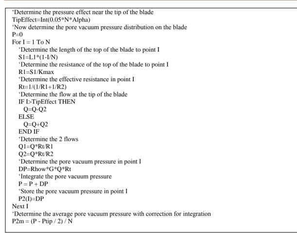
Figure 6-21: A small program to determine the pore pressures.
