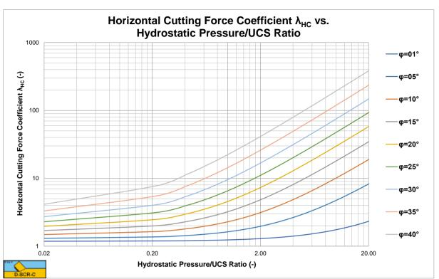
Figure X-13: The horizontal cutting force coefficient  $\lambda_{\rm HC}$  for a 60 degree blade.
