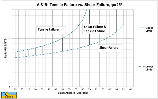
Figure W-22: The tensile/shear failure range based on UCS/BTS for  $\varphi$ =25°.
