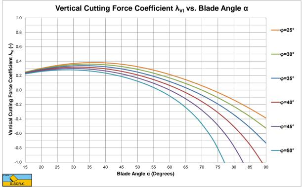
Figure B-26: The vertical cutting force coefficient  $\lambda_{VI}$  for a dimensionless inertial effect parameter  $\lambda_i$ =250.
