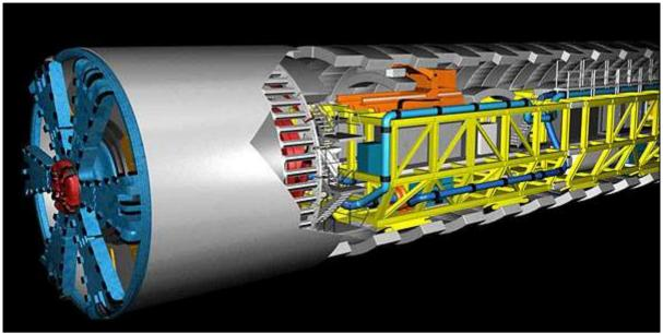
Figure Y-78: The WesterSchelde TBM.
