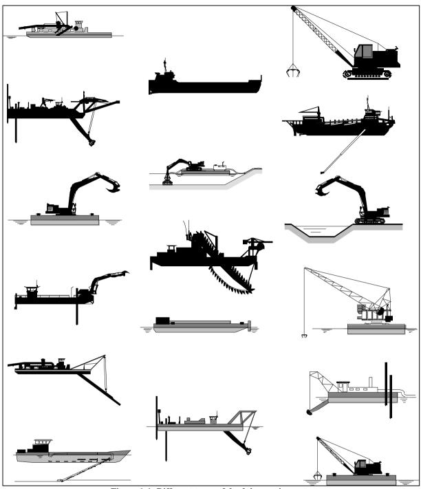
Figure 1-1: Different types of dredging equipment.
