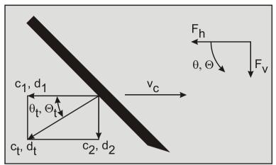
Figure 6-33: The total dimensionless cutting force ct, dt.
