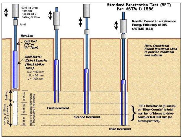
Figure 2-31: The Standard Penetration Test (www.shalviengineering.com).
