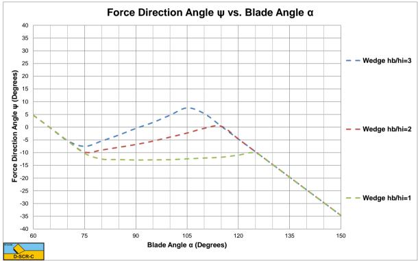
Figure 11-10: The direction of the total cutting force.
