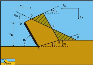
Figure 5-9: The alternative shape of the layer cut.
