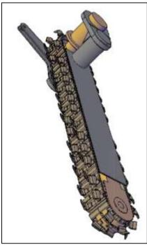
Figure Y-57: Arm with digging chain.
