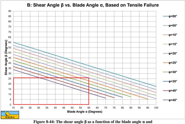
the internal friction angle φ.
