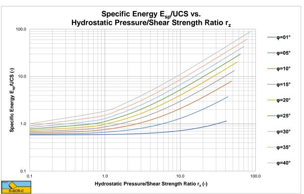
Figure 9-21: The E<sub>sp</sub>/UCS ratio, for a 60 degree blade.
