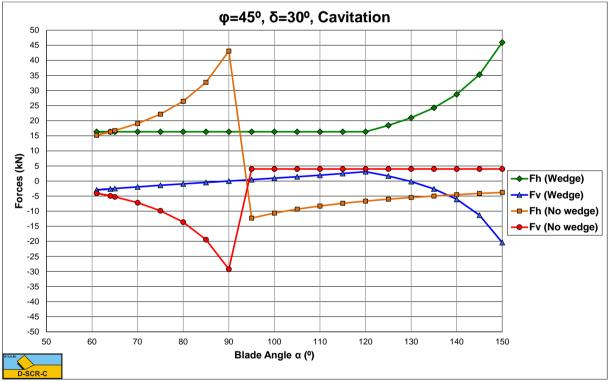
Figure Q-8: Cavitating, the cutting forces as a function of the blade angle  $\alpha$  for  $\varphi$ =45° and  $\delta$ =30°.
