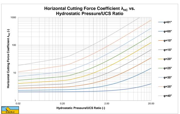
Figure X-23: The horizontal cutting force coefficient  $\lambda_{\rm HC}$  for a 90 degree blade.
