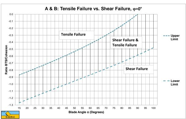
W.4 Transition Ranges Brittle Shear/Brittle Tensile.
