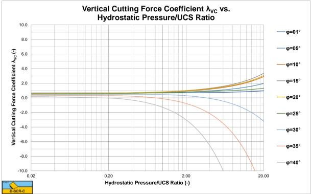
Figure X-14: The vertical cutting force coefficient  $\lambda_{\rm VC}$  for a 60 degree blade.
