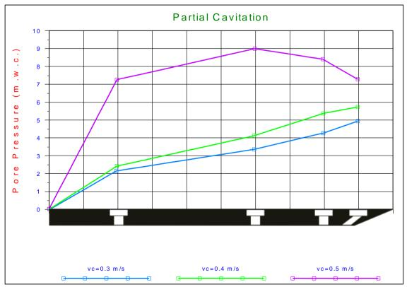
Figure M-2: Measured absolute pore pressures.
