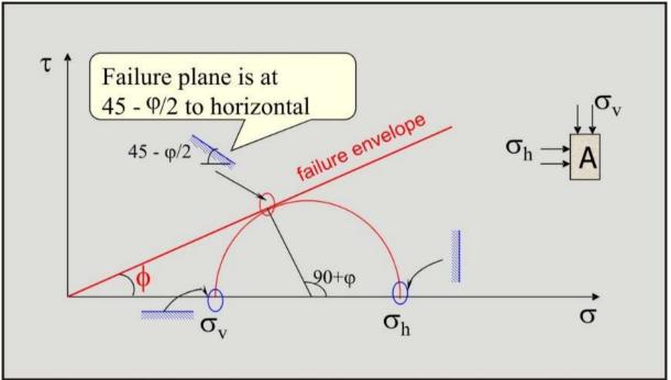
Figure 2-55: The Mohr circle for passive soil failure.
