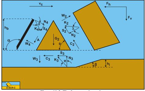
Figure 10-3: The forces on the wedge.
