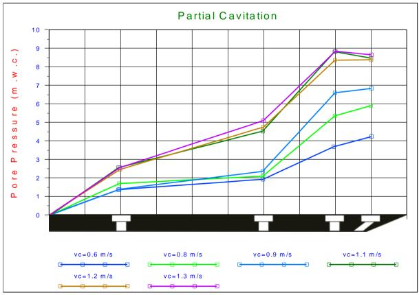
Figure M-8: Measured absolute pore pressures.
