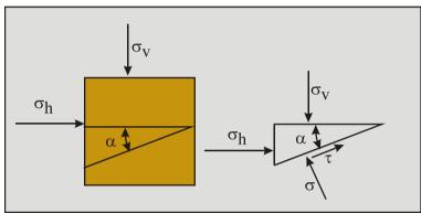
Figure 2-44: The stresses on a soil element.
