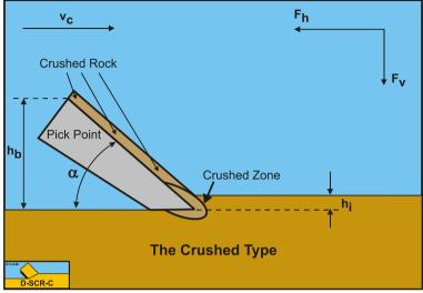
Figure 4-6: The Crushed Type in atmospheric rock cutting.
