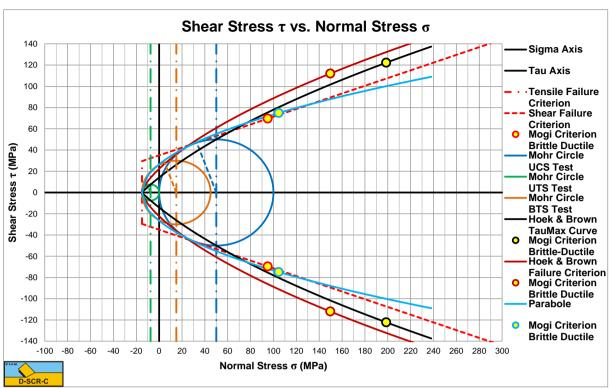
Figure 8-17: The failure criteria.
