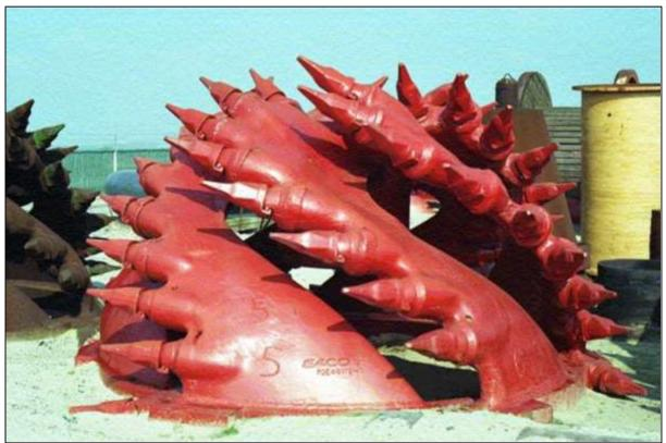
Figure Y-16: Rock cutterhead (IHC).
