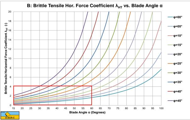
Figure W-36: The brittle (tensile failure) horizontal force coefficient  $\lambda_{HT}$ , corrected.
