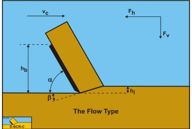
Figure 4-4: The Flow Type in clay and loam cutting.
