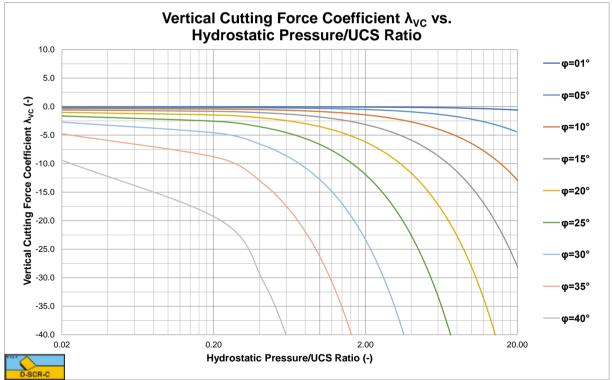
Figure X-24: The vertical cutting force coefficient  $\lambda_{\rm VC}$  for a 90 degree blade.
