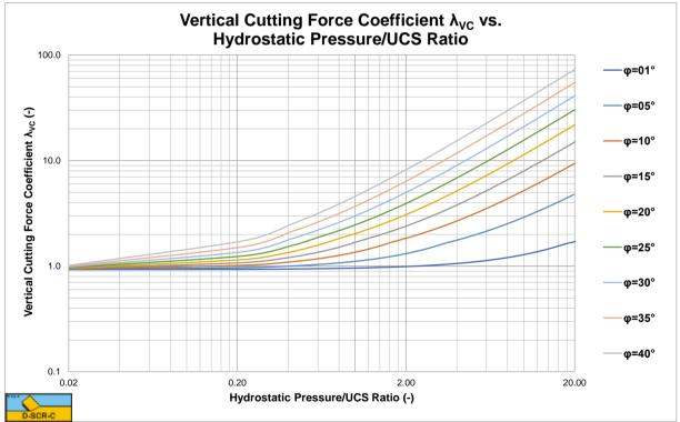
Figure X-4: The vertical cutting force coefficient  $\lambda_{\rm VC}$  for a 30 degree blade.
