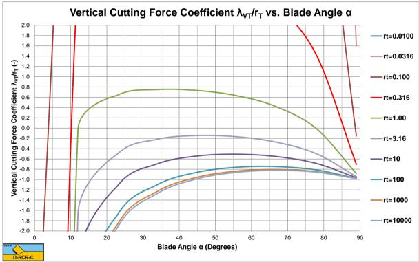
Figure 7-32: The vertical cutting force coefficient  $\lambda_{\rm VT}/r_T$  zoomed.
