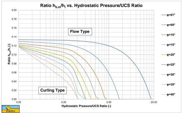
Figure X-1: The ratio h<sub>b,m</sub>/h<sub>i</sub> for a 30 degree blade.
