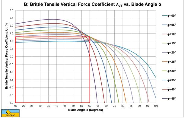
Figure 8-46: The brittle (tensile failure) vertical force coefficient  $\lambda_{\rm VT}.$
