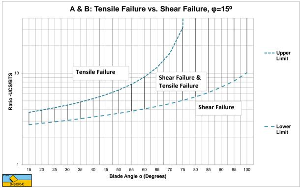
Figure W-18: The tensile/shear failure range based on UCS/BTS for  $\varphi$ =15°.
