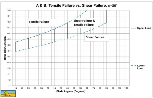
Figure W-23: The tensile/shear failure range based on BTS/Cohesion for  $\varphi$ =30°.
