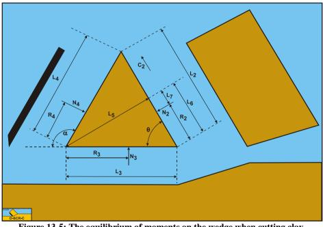
Figure 13-5: The equilibrium of moments on the wedge when cutting clay.
