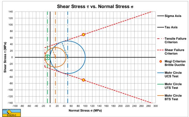
Figure 8-16: The linear failure criterion.
