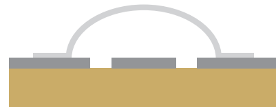
Figure 3.5: Schematic of the fabrication process. There are 4 electron beam lithography steps: one for the definition of the base-layer features, one for the definition of the Josephson junctions and two for the airbridge crossovers. Only the Josephson junctions require nanometer precision, the other steps could in principle be done with optical lithography.
