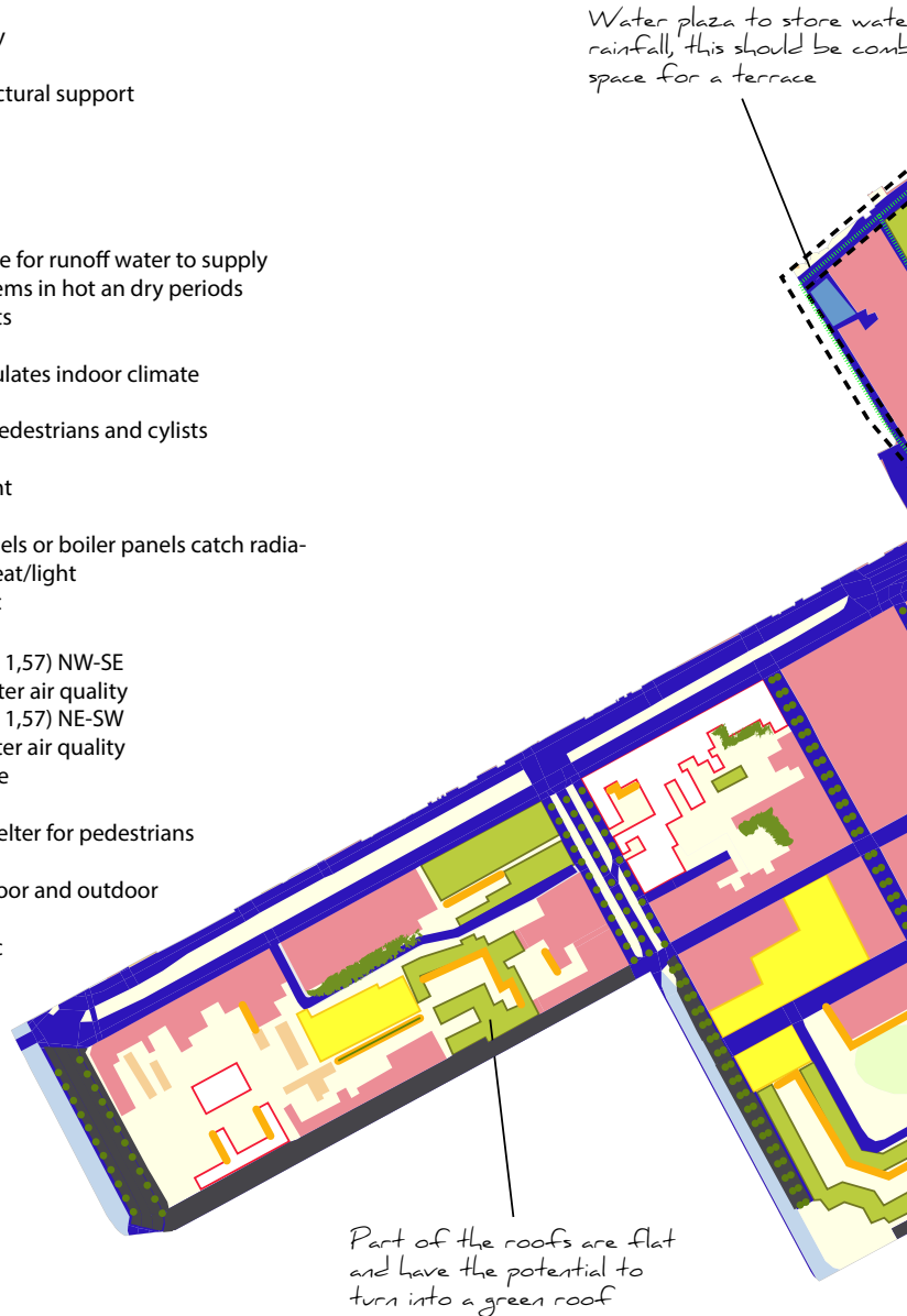
FIGURE 9.15 The Zuidwal neighbourhood in The Hague with a wide range of climate adaptation measures to improve thermal comfort on hot days.
