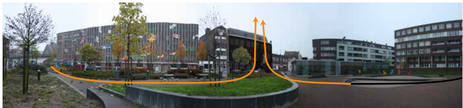
FIGURE 9.28 Expected thermal induced air currents with a dark façade of the old chocolate factory at the Insulindeplein
