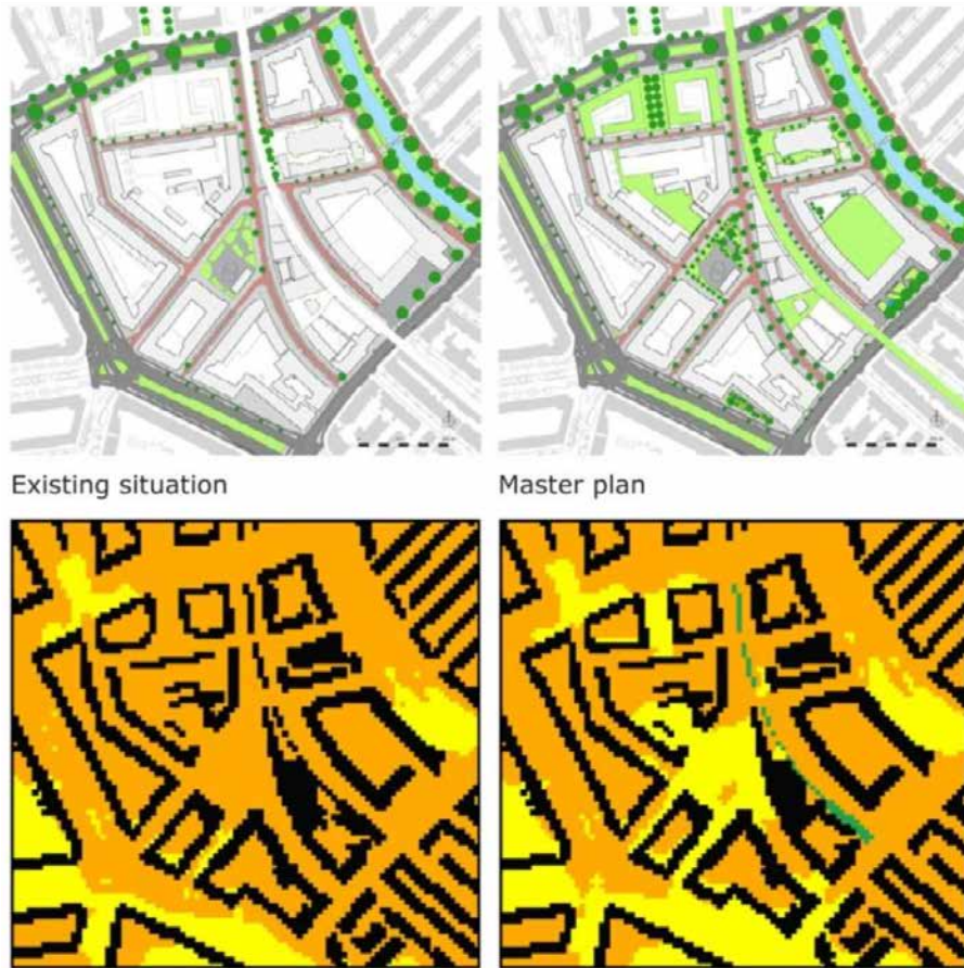
FIGURE 9.23 Simulation results by ENVI-met in potential air temperature for 7-8-2013, 13:00h at a height of two meters. Yellow indicates 25.5-26°C and orange 26-26.5°C (Kleerekoper et al., 2012).
