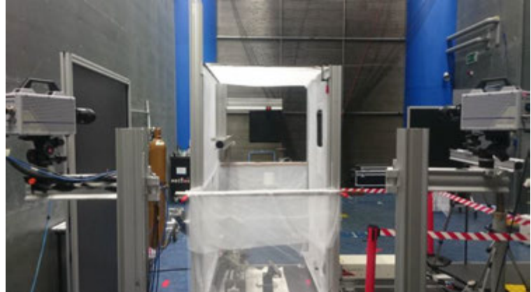
Fig. 5. Top view schematic of the test arrangement (left); setup for the stereoscopic PIV measurements (right).
