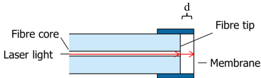
Figure 2.4 Schematic representation of a fibre tip with an eFPI sensor, where d is the distance to the membrane creating a cavity.
