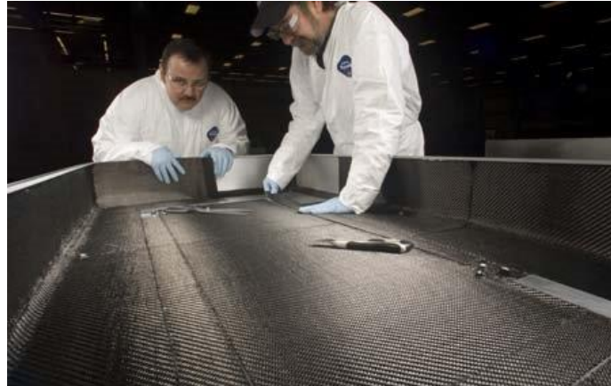
Figure 1.3 An example of hand layup, where workers apply CFRP layers to a mould. (© Lee Aerospace)
