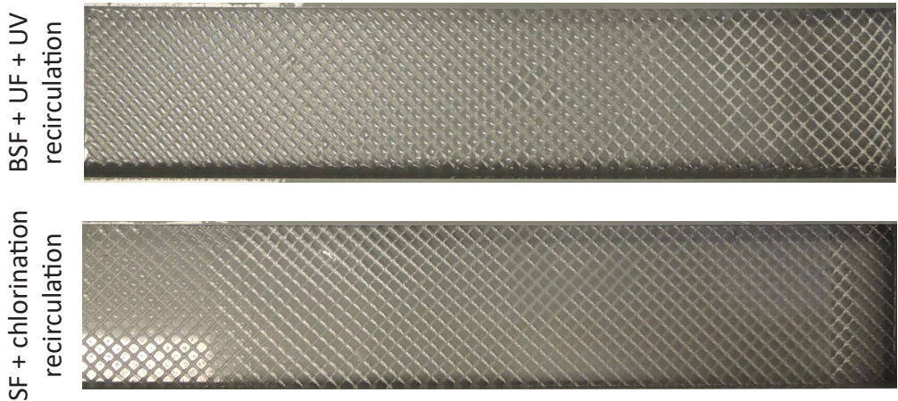
Figure S5: Membrane spacer inside MFS units at recirculation conditions after 23 d duration. Flow direction was left to right.
