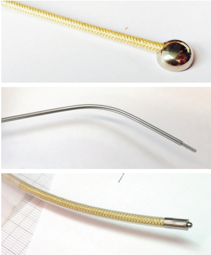
Figure 6. Three categories of prototypes that have been developed. Top: compliant tubing equipped with a disc shaped nozzle to provide stability during water jet drilling and counteract potential damage to the opposite cartilage surface. Center: rigid tubing, allowing the instrument to be smaller than 2 mm in diameter. Bottom: compliant tubing equipped with a 9 mm long rigid nozzle.
