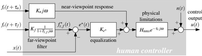
Fig. 2. Quasi-linear human controller model for preview tracking tasks with integrator controlled element dynamics [8]. The near-viewpoint response dynamics are simplified, in accordance with [9].
