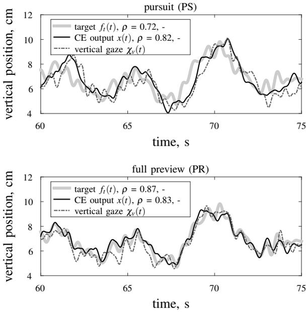
Fig. 8. Vertical gaze position, target, and CE output time-traces from a run where the gaze data were relatively low noise. The Pearson correlation coefficients  $\rho$  indicate the signals' correlation with the vertical gaze position.
