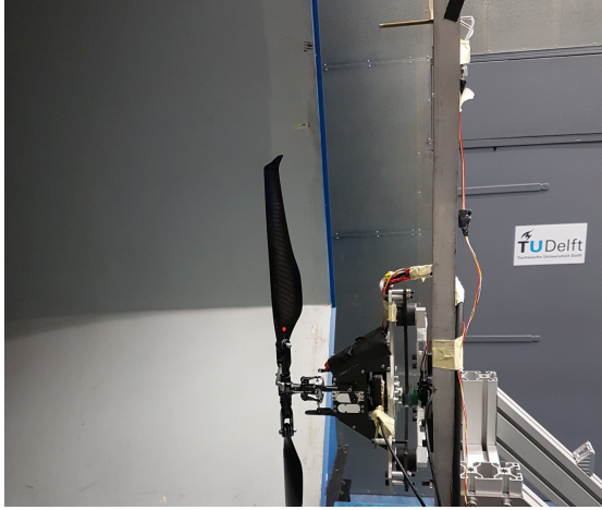
Figure 2: Close up of the new rotor blades (left), the force and moment balance (middle) and the airspeed probe (on top). The windtunnel blows from left to right.
