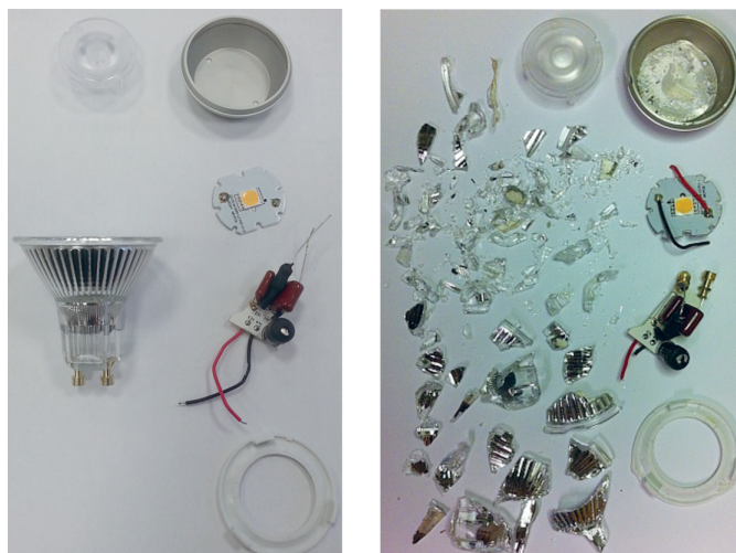
Figure 4.10-Redesigned spot lamp with glass housing, before and after shredding. Images provided by Johan Felix, CIT Recycling Development AB.
