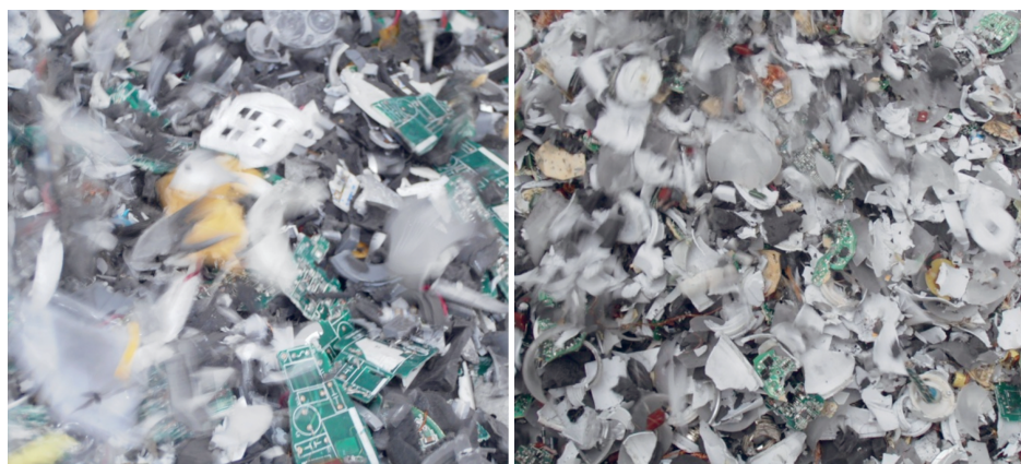
Figure 3.23-Low-density fraction after wind sieve separation for LED bulbs in Run1. Left: spots, right: bulbs. Images provided by Johan Felix, CIT Recycling Development AB.
