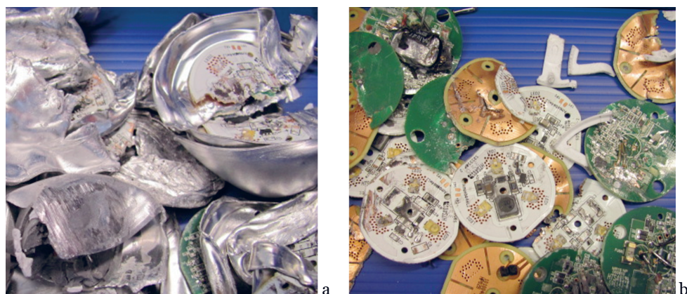
Figure 4.8- a: fragments obtained from shredding of staked LED spot lamps, b: PCB fragments after shredding when potting is added. Images provided by Johan Felix, CIT Recycling Development AB.
