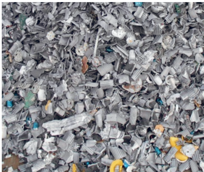
Figure 3.20-Aluminium fraction after eddy current separation for spots LED lamps. Image provided by Johan Felix, CIT Recycling Development AB.
