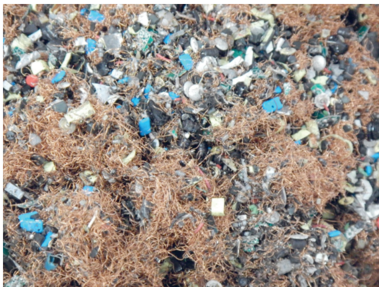
Figure 3.24-Metal-rich high-density fraction obtained from Run 2. Image provided by Johan Felix, CIT Recycling Development AB.
